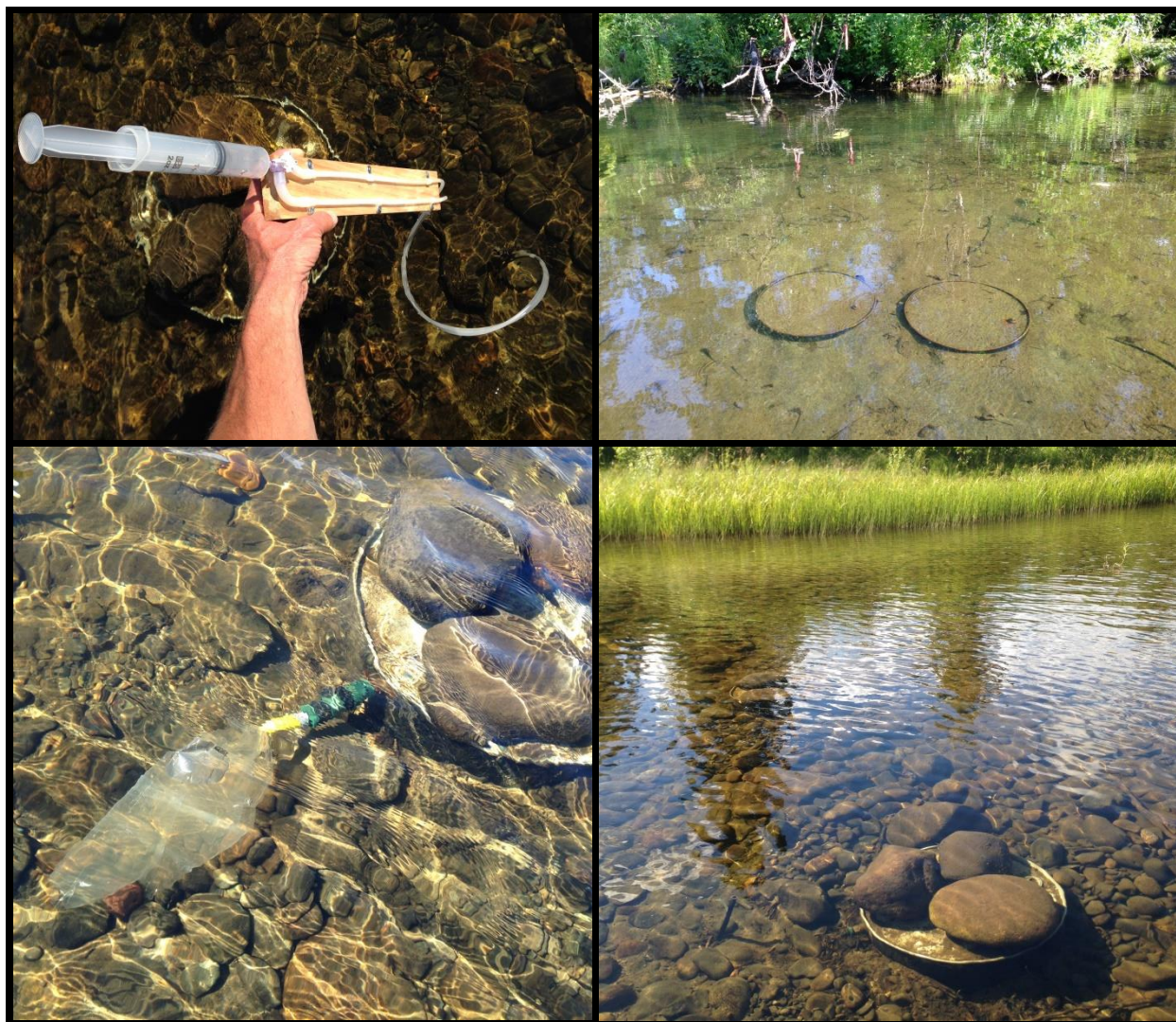
Figure 2.4.1-6. Representative photographs of seepage meter installations during summer 2016.
