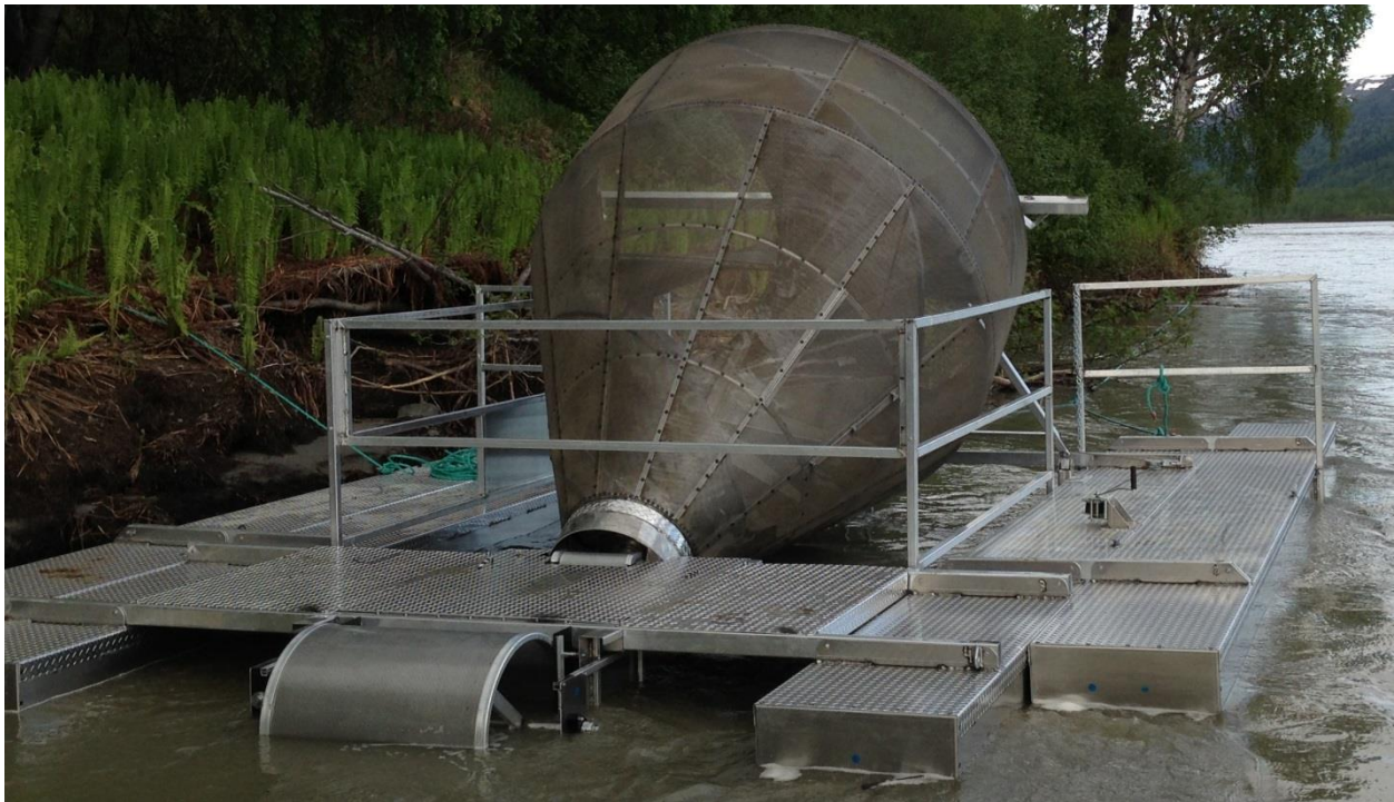
Figure 2.6.1-7. Photo of rotary screw trap used on the Susitna River with fine mesh debris drum.
