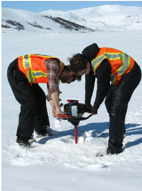
Figure 4.1-2: Augering a hole in the over 1 m thick ice at Big Lake.
