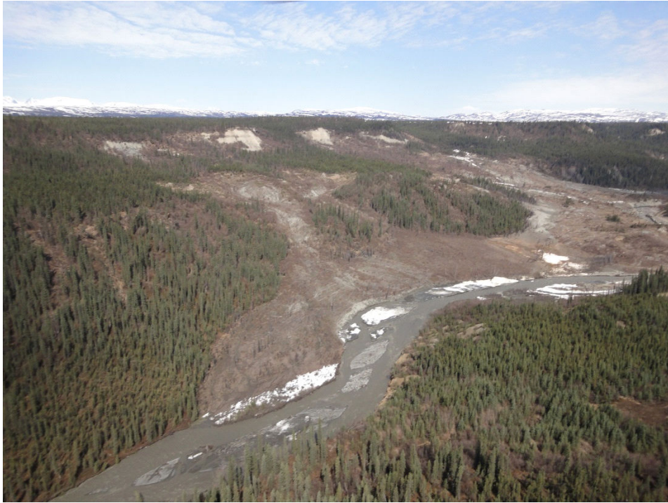
Figure 10. Translational Slide on SW-facing Slope along Watana Creek (Sheet 12-5).
