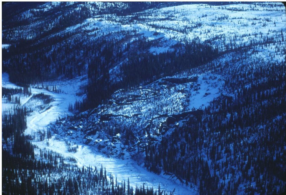
Figure 11. Translational Slide, Earth Block Slide of Frozen Ground, NE-facing Slope, Watana Creek (Sheet 12-6).
