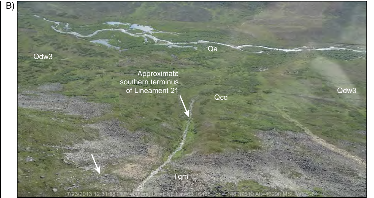
View looking southeast from photograph location B. Arrows show the projected trace of Feature 21 lineament.
