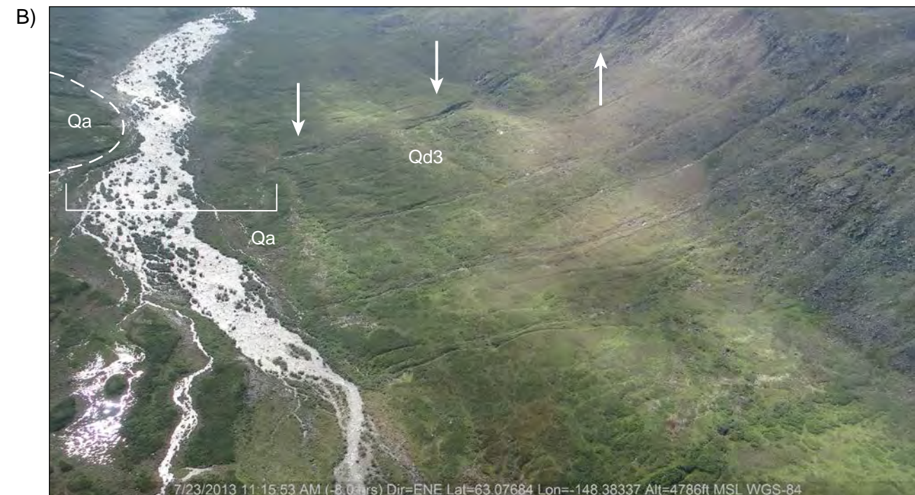
View looking south from photograph location B. Arrows show the projected trace of lineament. In Qd3 (till) the lineament is coincident with linear drainage in till deposit. Note absence of lineament in Qa deposit.
