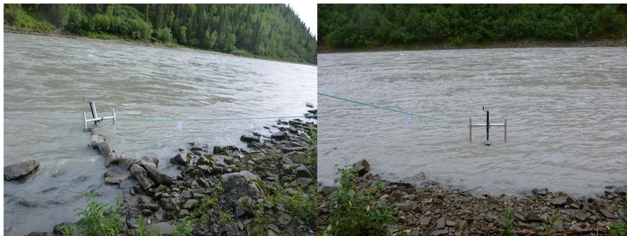
Figure G-2. Photographs showing the ARIS mounts deployed at the left bank (left) and right bank (right) monitoring stations.
