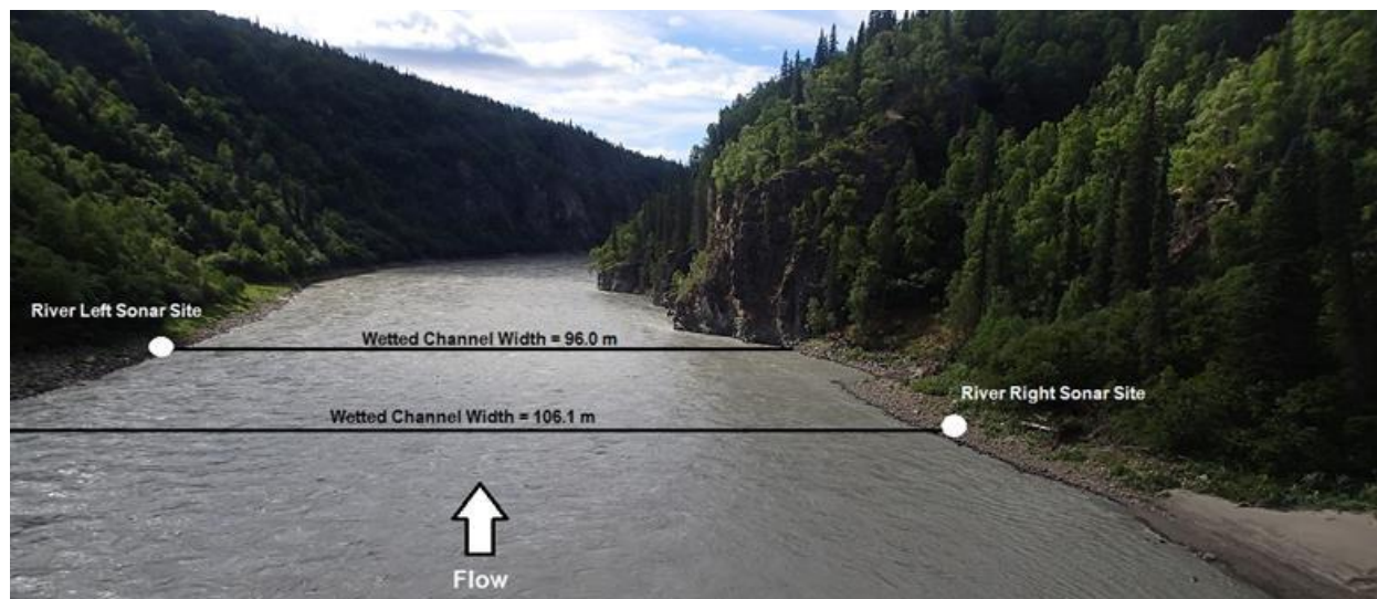
Figure G-1. Photograph of the Susitna River immediately downstream of the proposed Watana Dam Site (PRM 187.1) showing the location of the river left and river right sonar sites and the wetted channel width.
