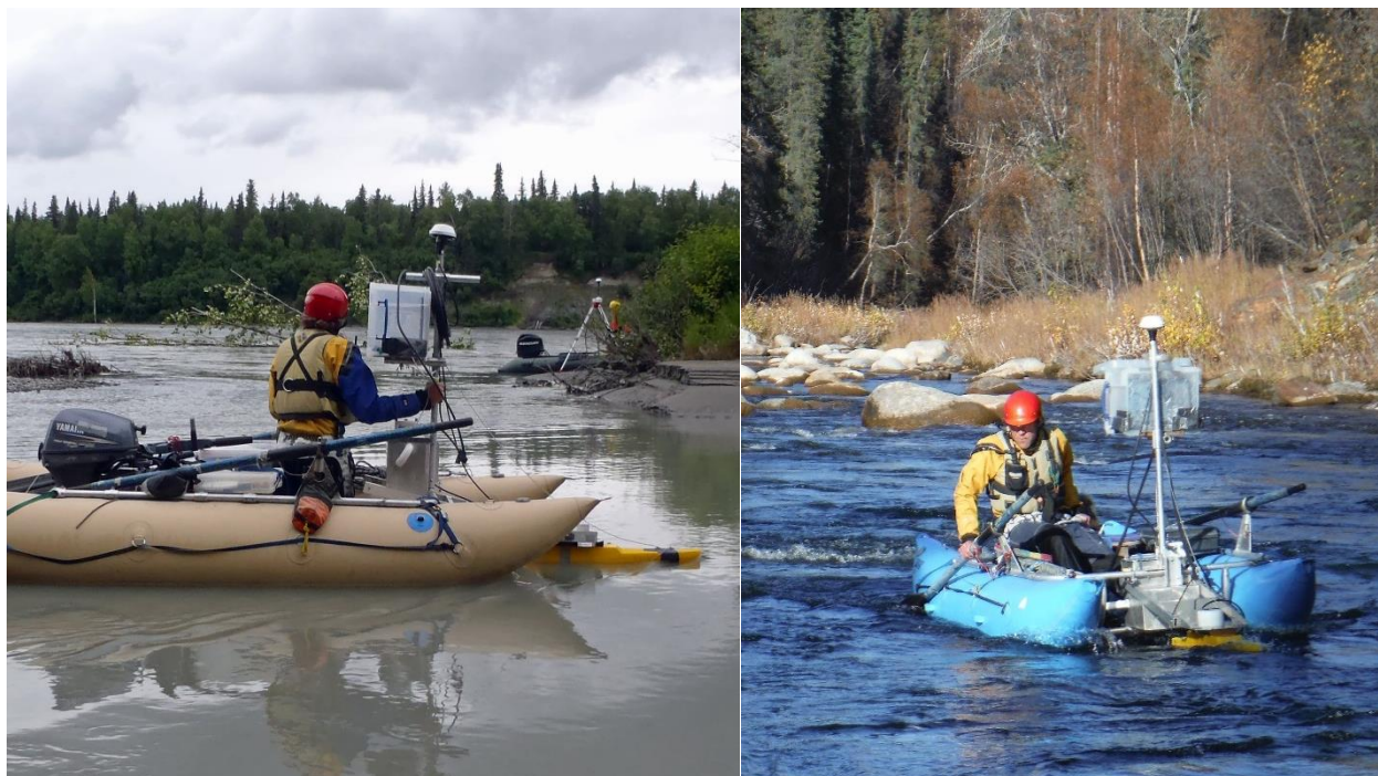
Figure 3. Techniques for maintaining a constant boat orientation.
