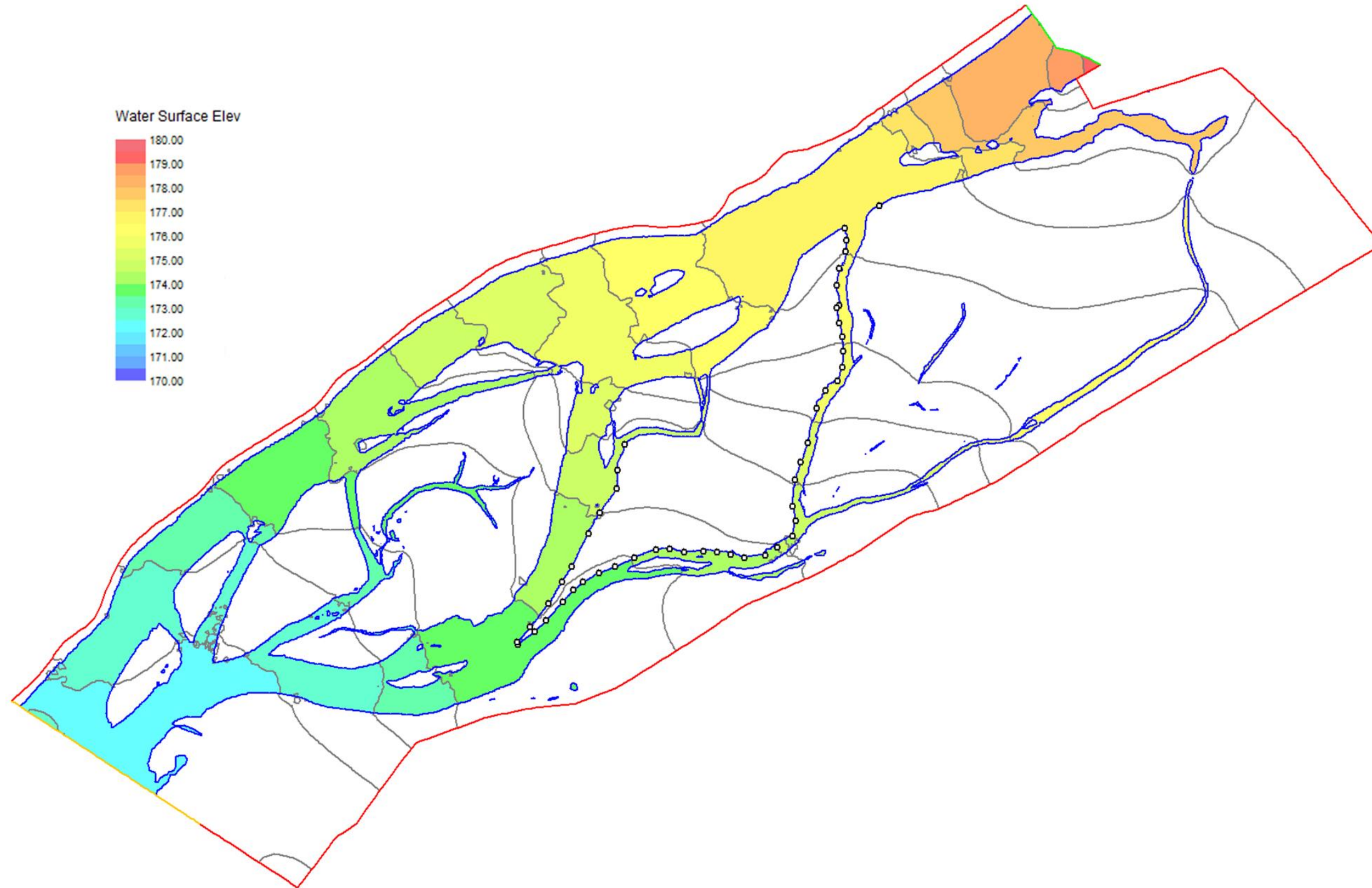
Figure 6. Slough 8A Complex (FA-128) River2D surface-water elevation (in meters) and water-edge survey locations (open circles) for the June 28, 2013 calibration. Grey contour lines are in 0.5-meter increments
