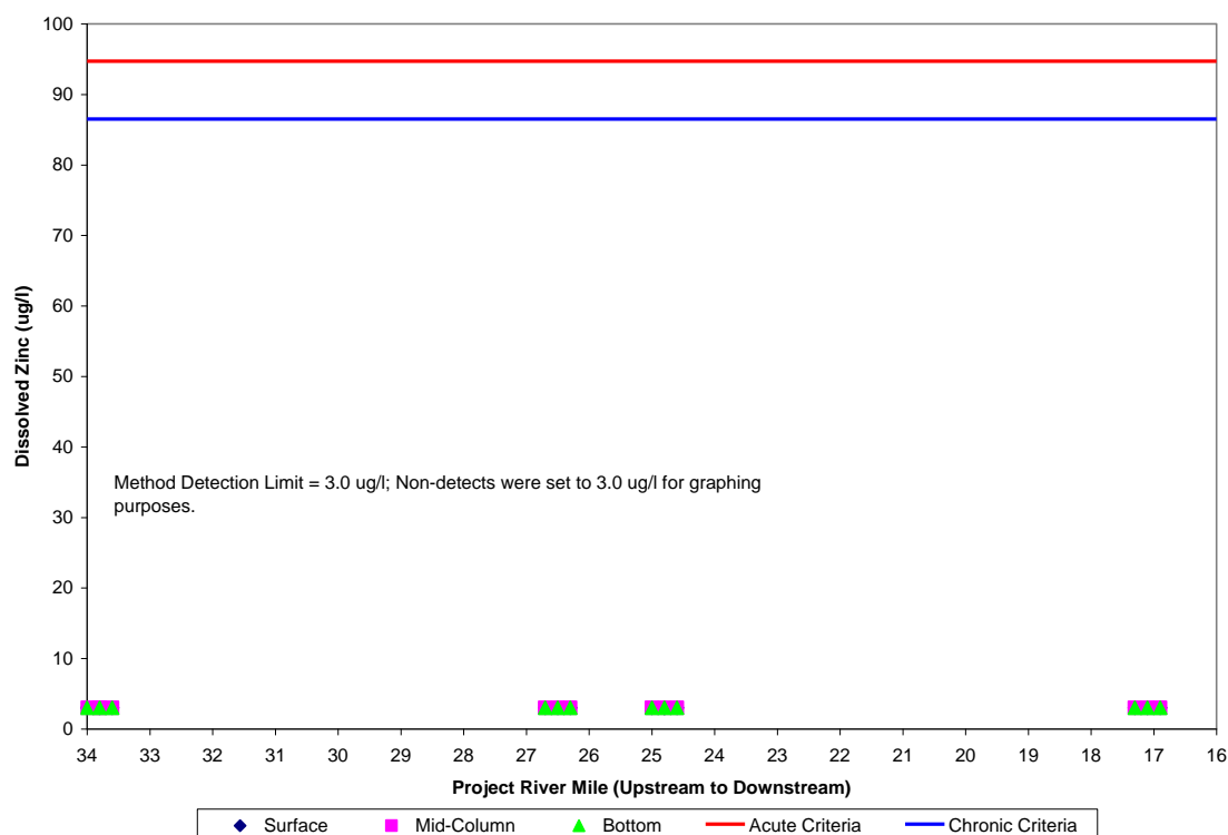
Figure 5-3. Example of water column samples collected from multiple sediment sampling sites and zinc concentration in each (note the water quality criteria inserted into the graph).
