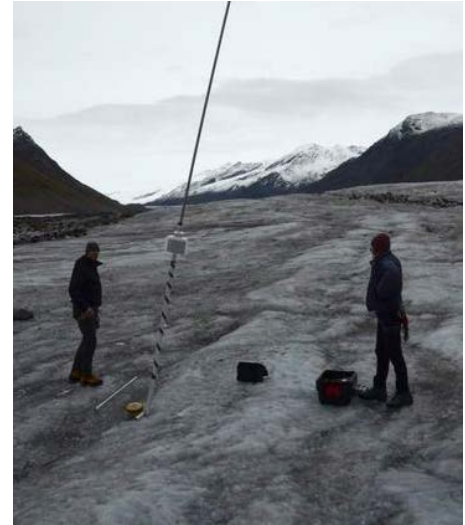
Figure 5.3.7-2. The design of the glacier weather monitoring stations allowed the sensors to remain at approximately the same height relative to the glacier surface throughout the melt season.
