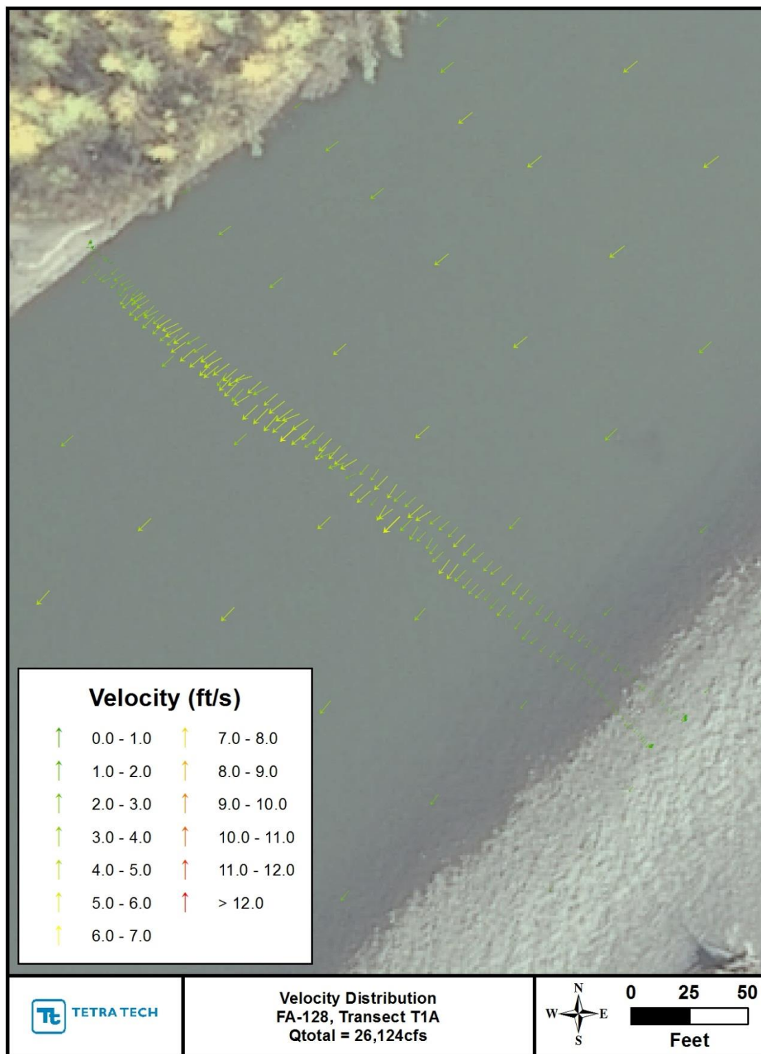
Figure 2.3-19. Comparison of measured and predicted velocity magnitude and direction at Transect 1A (Figure 2.2-7) at 26,184 cfs (Sept. 10, 2013).
