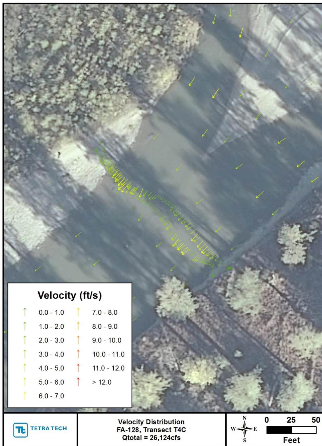
Figure 2.3-24. Comparison of measured and predicted velocity magnitude and direction at Transect 4C (Figure 2.2-7) at 26,184 cfs (Sept. 10, 2013).
