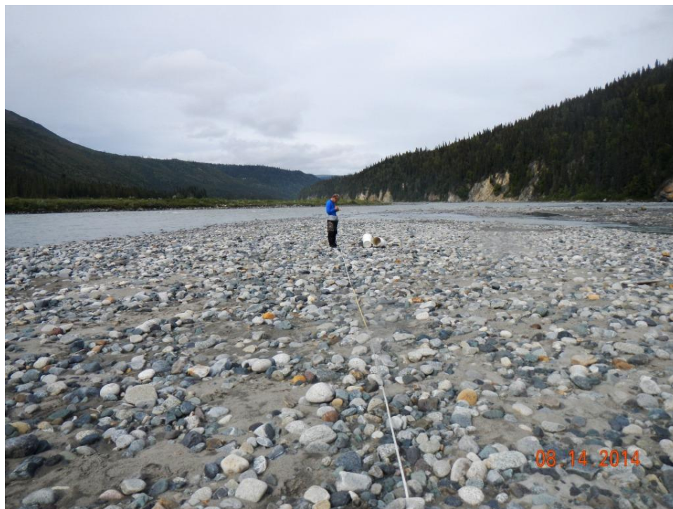
Figure A.2-50 – Imbricated surface material on gravel bar (PRM 224.6) in expansion zone downstream of Vee Canyon. Site of surface and subsurface sampling. Median particle diameter ( D_{50} ) of surface bed material is 68.3 mm. Median particle diameter ( D_{50} ) of subsurface bed material is 27.3 mm (P877).
