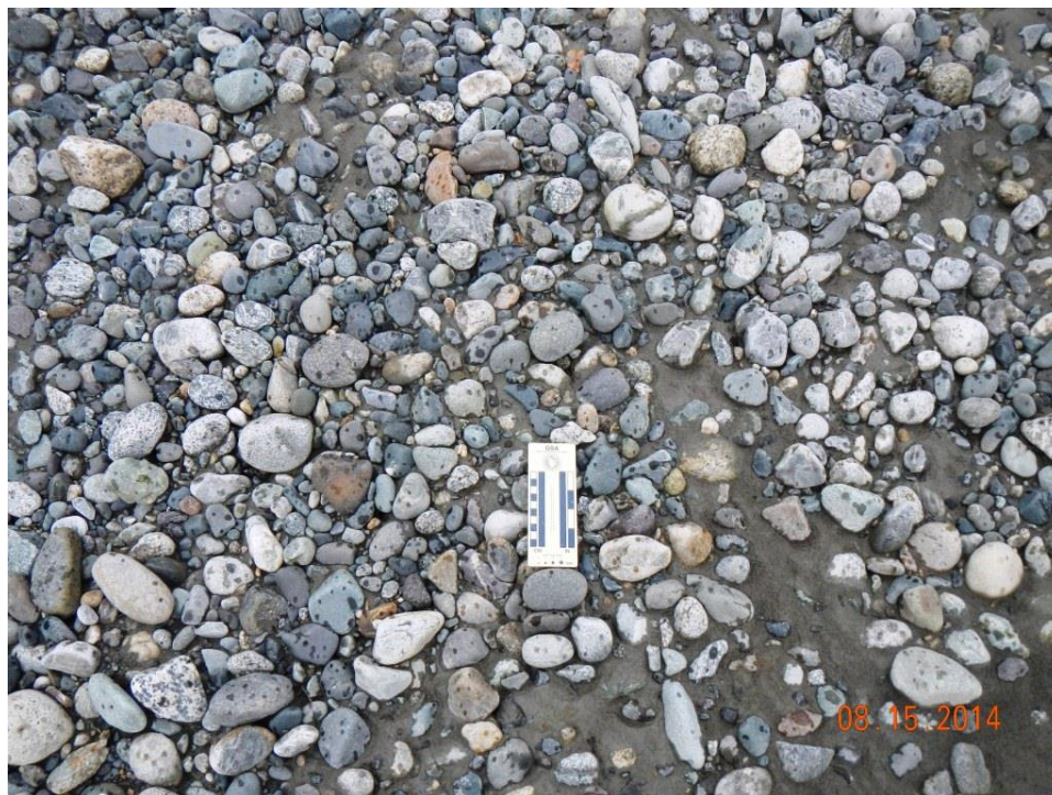
Figure A.2-71 – Surface material at PRM 206.8. Average median particle diameter ( D_{50} ) in reach (UR-5) is 47.5 mm (P165).
