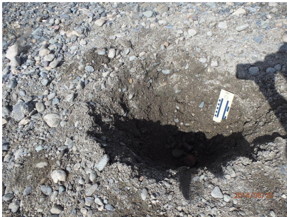
Figure A.2-5 – Surface and subsurface material at sediment sampling site at PRM 258.6. Median particle diameter ( D_{50} ) of surface sediment is 40.5 mm. Median particle diameter ( D_{50} ) of subsurface sediment is 10.1 mm (P821).
