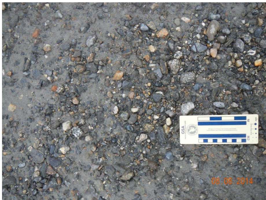
Figure A.1-3 – Surface material on mid-channel bar near PRM 291. Largest bar head particle diameter (b-axis) approximately 22mm (P774).
