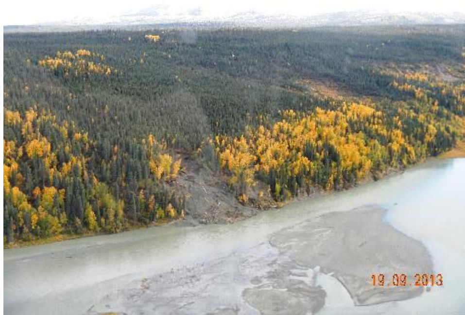
Figure A.2-82 - Active landslide in till near PRM 199.5 – Susitna River right bank (P5454).
