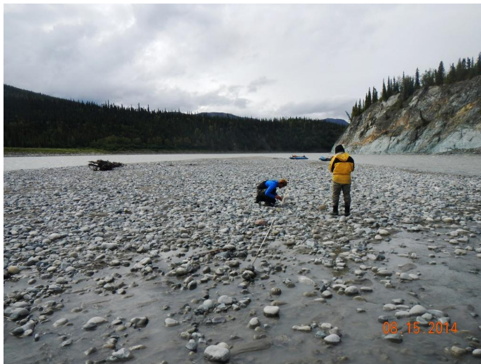
Figure A.2-66 – Surface material at head of bar at sediment sampling site at PRM 208.0. Bedrock outcrop on river right. Median particle diameter ( D_{50} ) is 47.5 mm (P127).
