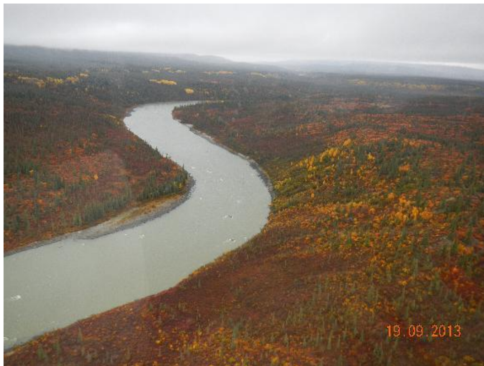
Figure A.2-32 – Confined channel with no islands or bars at PRM 240. Note large ice-deposited boulders in channel (indicated by surface disturbance in flow) (P5526).
