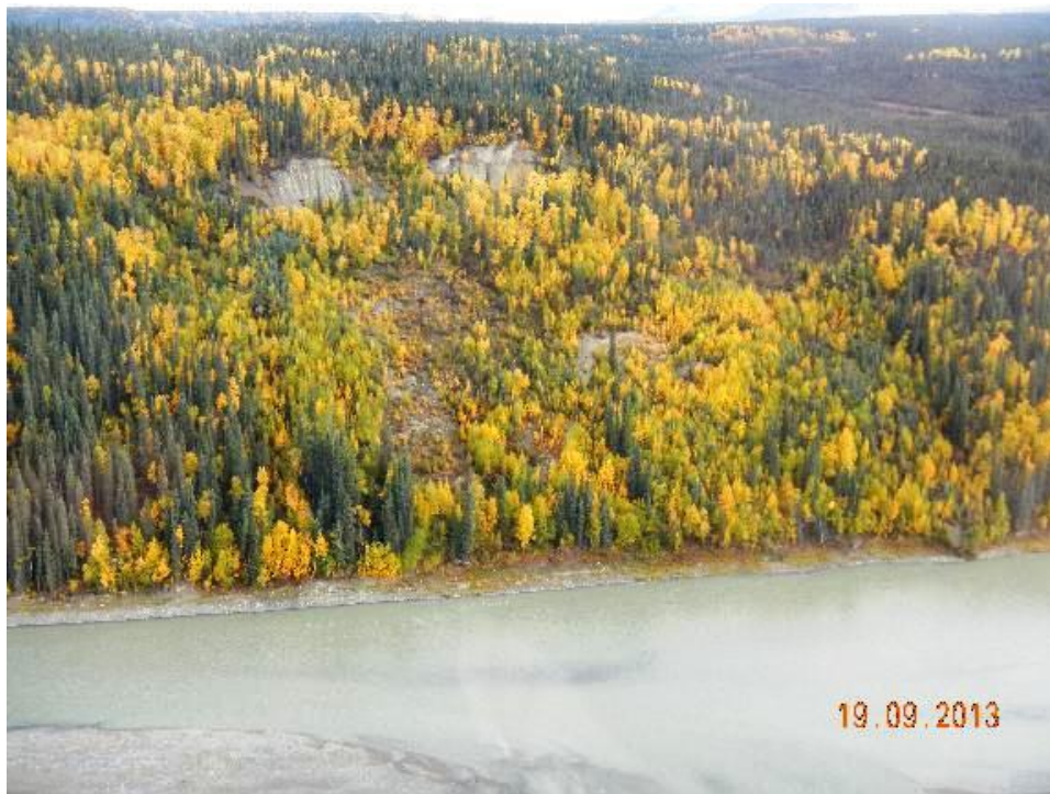
Figure A.2-85 – Active landslide in till near PRM 197.5 – Susitna River right bank (P5451).
