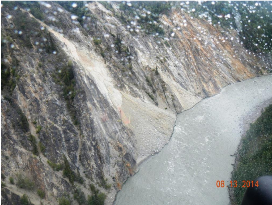
Figure A.2-47 – View upstream near PRM 226 at right bank colluvial cones in Vee Canyon – local bedrock source of large sediment (P757).
