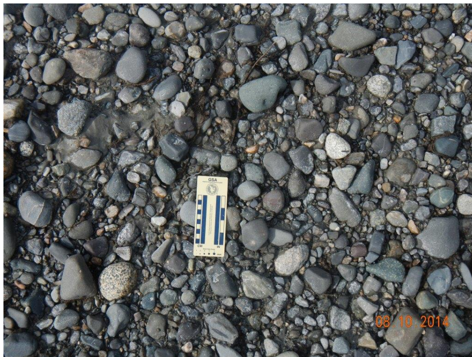
Figure A.1-29 – Gravel on mid-channel bar in expansion zone near PRM 266. Most gravel observed on the mid-channel bar ranged from 32 mm to 45 mm in diameter with some gravel sized at 64 mm to 90 mm (P082).
