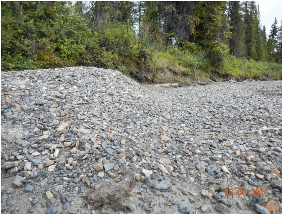
Figure A.1-9 – Fine gravel lobes at PRM 276.2. Grab sample location - median bed material diameter ( D_{50} ) is 4.2 mm (P927).
