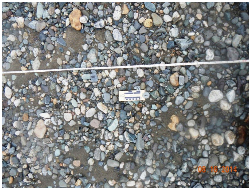
Figure A.2-88 – Surface material at sediment sample location at PRM 196.5 – first exposed mid-channel bar downstream of Watana Creek. Median particle diameter ( D_{50} ) is 26.1 mm (P374).
