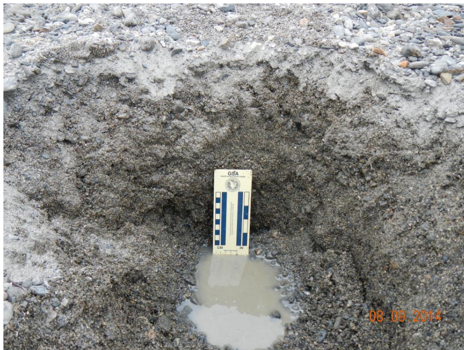
Figure A.1-13 – Subsurface material on alternate bar at PRM 276.2. Grab sample location - median bed material diameter ( D_{50} ) is 4.2 mm (P935).
