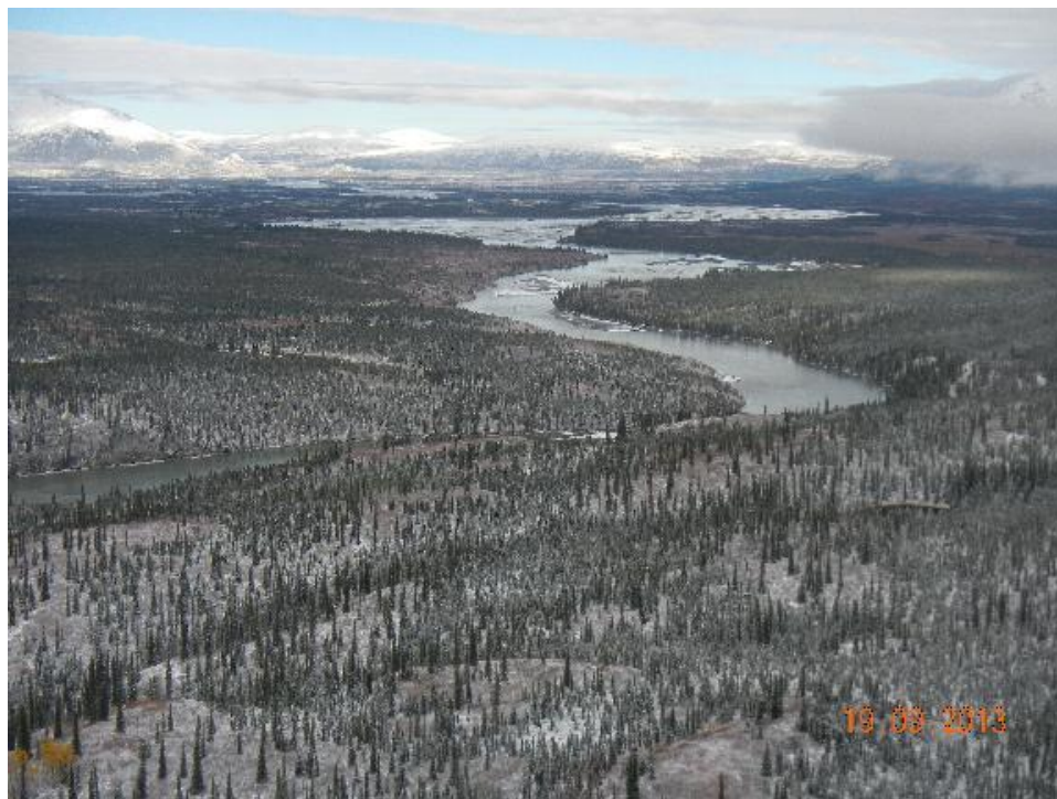
Figure A.1-16 – View upstream at PRM 274. Forced sinuosity due to presence of tills and bedrock (P5559).
