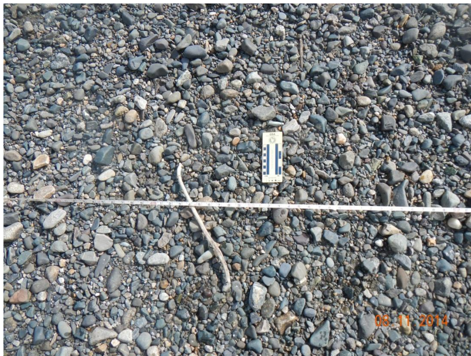
Figure A.2-19 – Surface material on bar surface at PRM 250.9. Median particle diameter ( D_{50} ) is 30.0 mm (P425).
