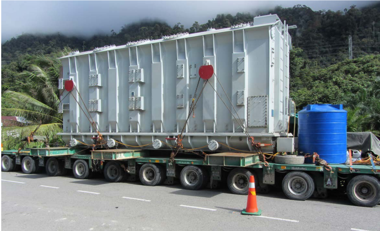
Figure 13.3-9. Transformer Transport by Road
