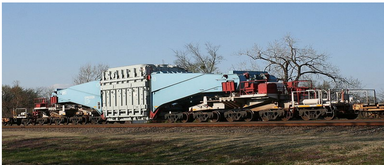
Figure 13.3-8. Transformer Transport by Rail
