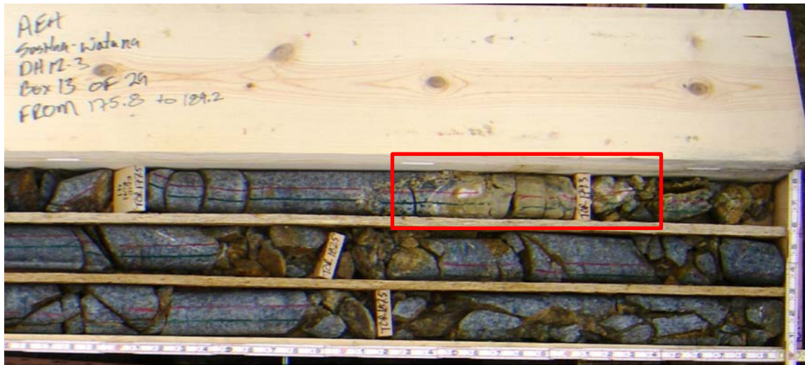
Figure 6.3-22. Rock Core from DH12-3 with Closely Fractured Rock and Shear Zone at Depth of about 179 ft. (red box)
