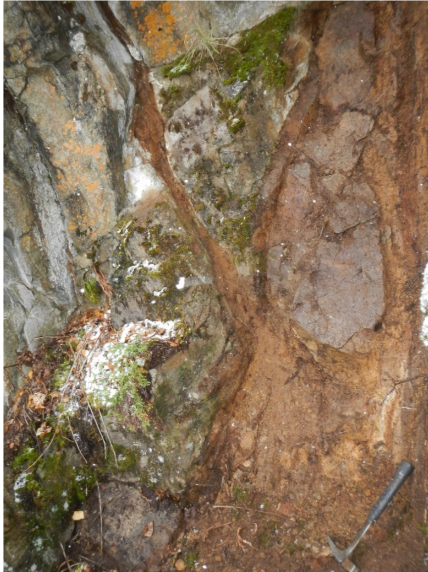
Figure 6.3-31. Shear Zone near BS 36, Main Shear Zone on Right with Inclined Shear Zone Splay
