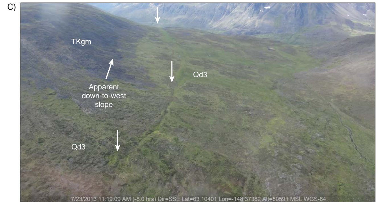
View looking south from photograph location C. Arrows show the projected trace of lineament. Note lineament is coincident with a linear drainage in this view.
