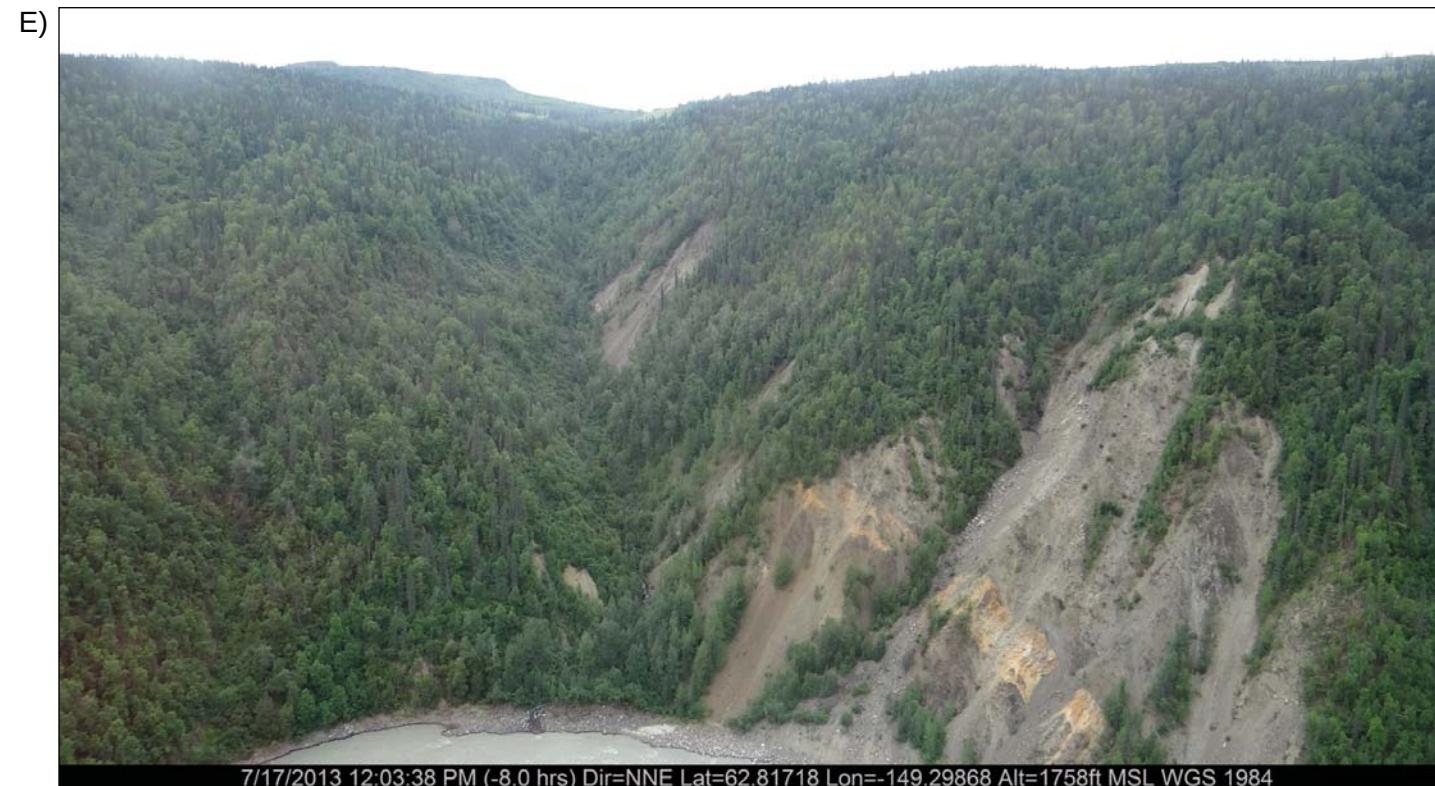
View looking north at north (right) bank of Susitna River showing oxidized mafic dike interpreted by WCC (1982) to not be truncated by the linear drainage.
