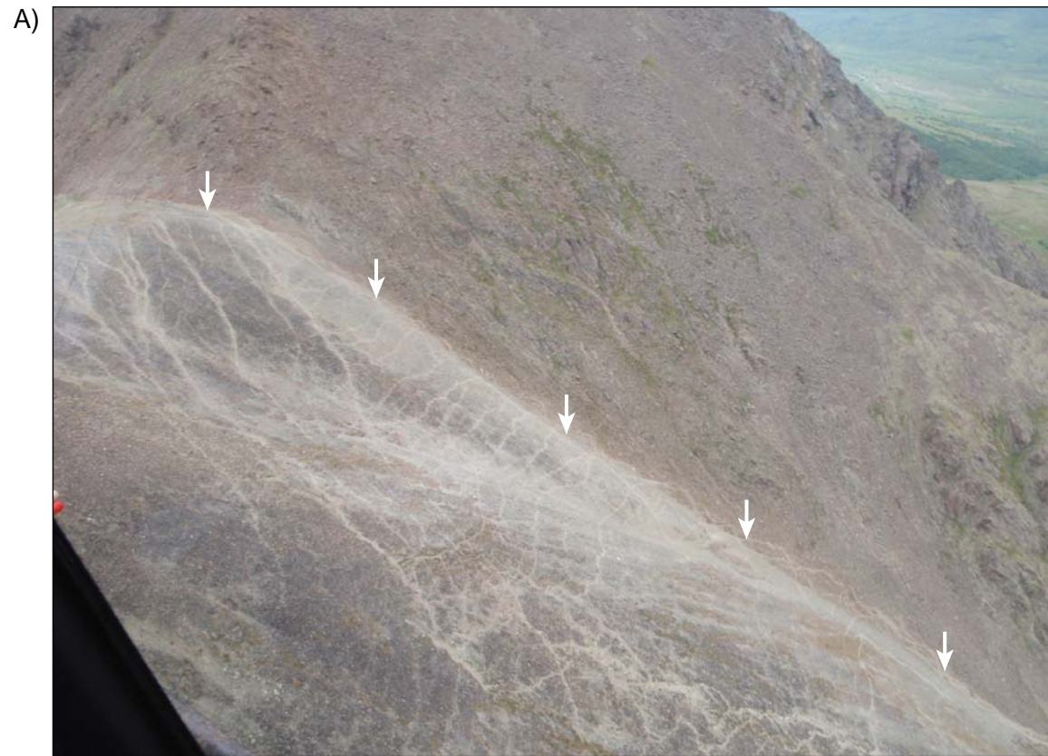
View looking at color contrast at previously mapped bedrock fault.
