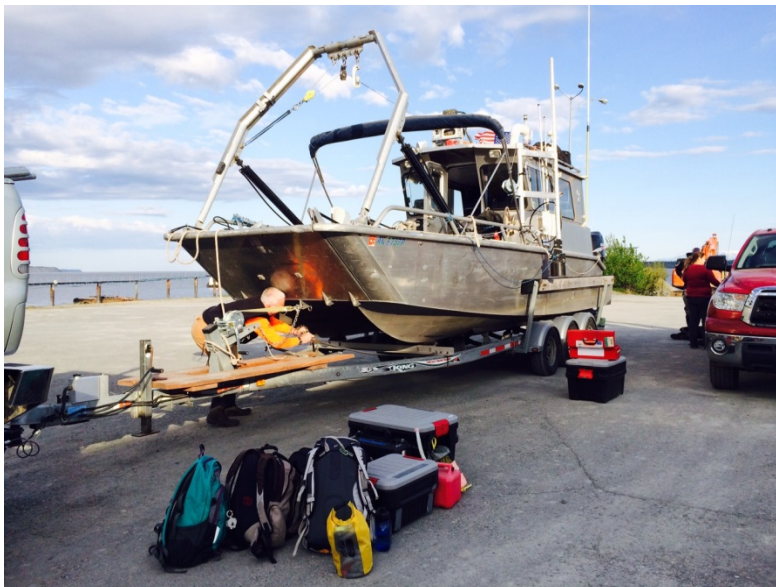
Figure 1. Landing craft used for surveys. The mounted transducer is on the port side of the vessel forward of the wheelhouse.
