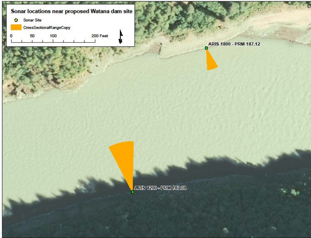
Figure 4.3-1. Ortho image showing the ensonified wetted width coverage of each ARIS unit near the Watana Dam Site, 2014. Ensonified coverage is scaled to match the width of the river. River flow is from right to left.
