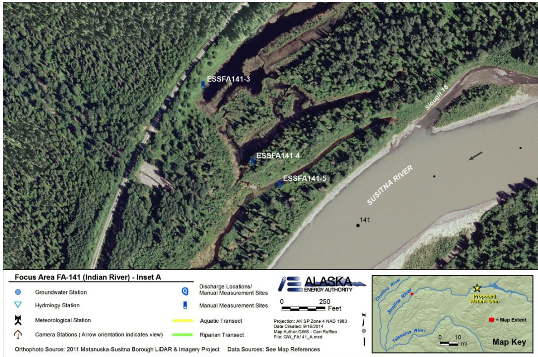
Figure 6. Inset A shows locations of aquatic transect stations with continuously measured parameters at FA-141 (Indian River) Focus Area.
