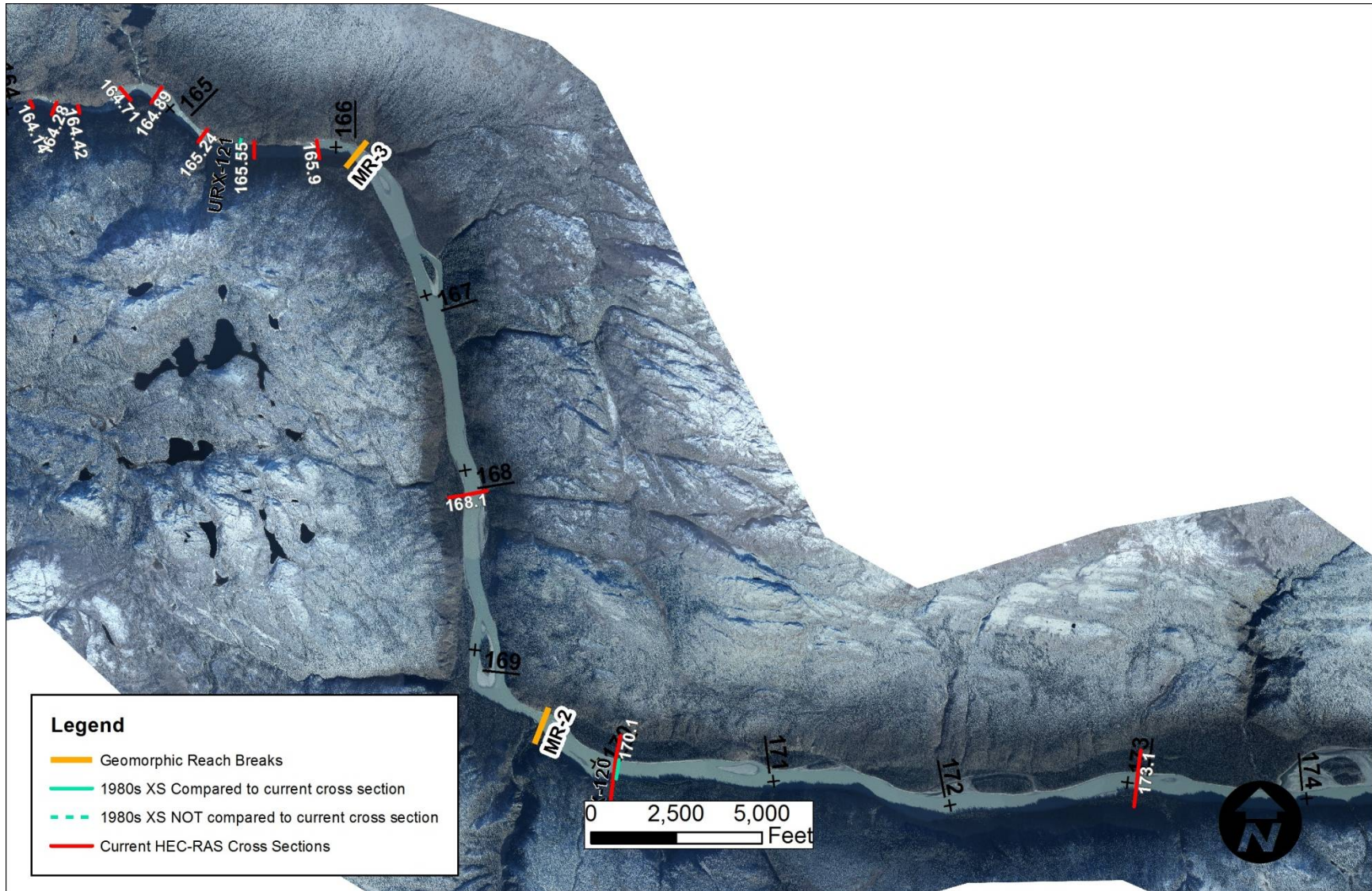
Figure 4.3-3 Cross section locations for 1980s HEC-2 cross sections and current HEC-RAS cross sections from PRM 174 to PRM 164.
