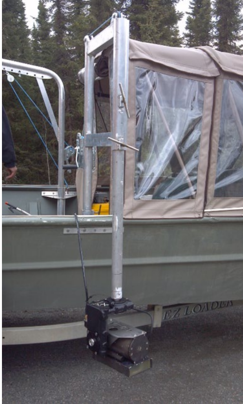
Figure 4.2-3. DIDSON imaging sonar and X2 rotator deployed over the side of the boat in 2013.
