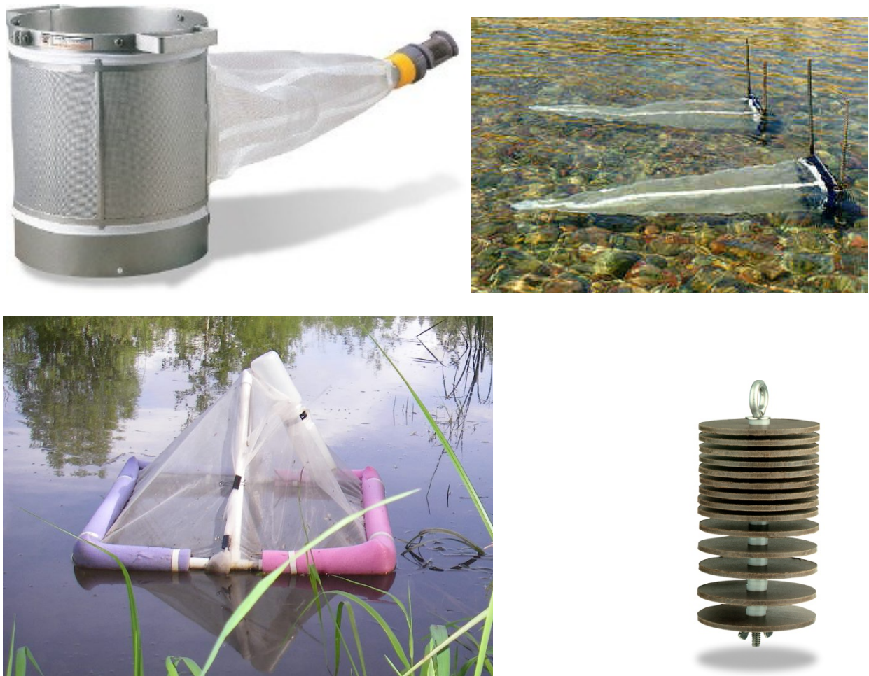
Figure 4.4-1. Sampling equipment used to collect benthic macroinvertebrates in streams and rivers. Top left: Hess stream sampler. Top right: drift nets. Bottom left: floating aquatic insect emergence trap. Bottom right: Hester-Dendy multiplate sampler.
