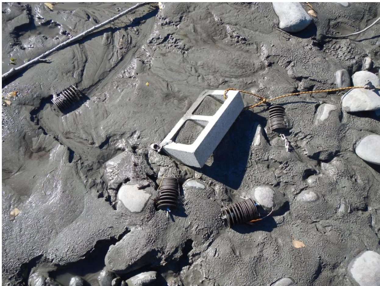
Figure 4.11-1. Hester-Dendy multiplate sampler set retrieved at RP-HD-3 on September 20, 2013. Declining flows over the previous week resulted in both large amounts of sediment deposited at the site, which was then dewatered.
