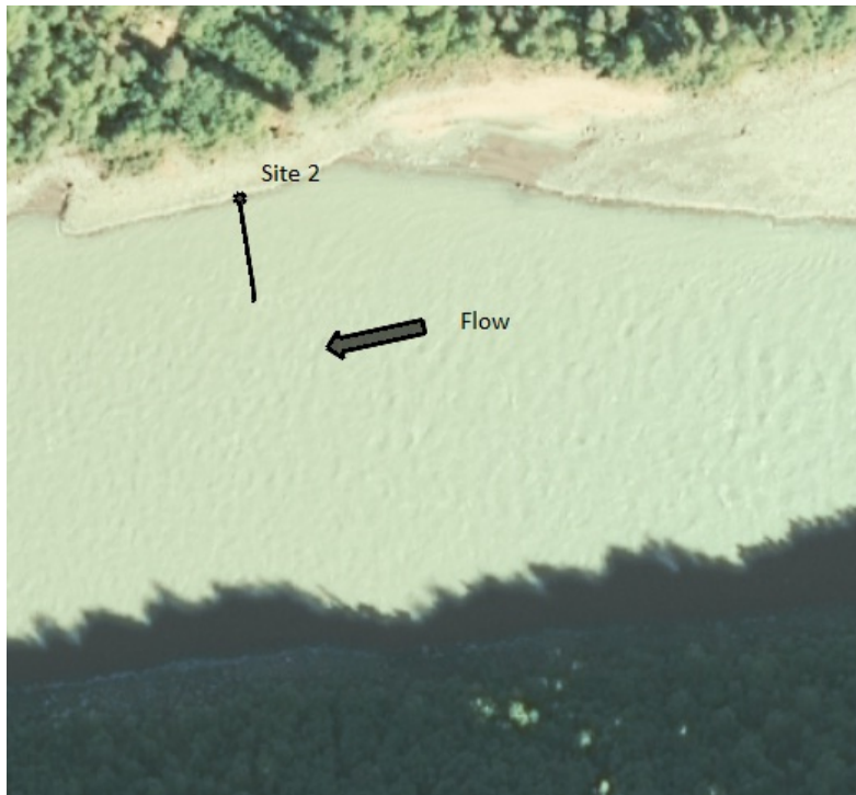
Photo G-5. Ortho-rectified aerial photographs of Site 2 assessed for sonar monitoring suitability in the Watana Canyon reach of the Susitna River, 2013. The line projecting from the sample site location depicts the effective range (20 m [65 ft]) of the sonar tested during the feasibility study.
