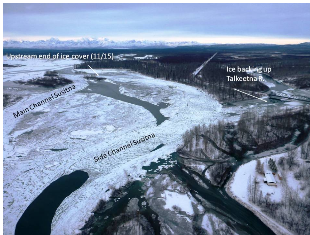
Figure 2.1-7. PRM 100-102 (RM 96.6-98.2) - Ice cover configuration and flooded channels at Talkeetna. November 15th, 2012.
