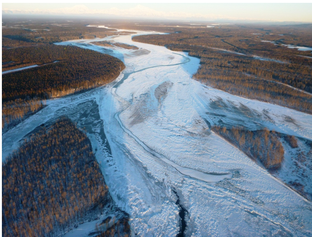
Figure 2.1-3. PRM 78 (RM 74.3) - Looking upstream. Velocity lead in main channel filling in from bottom with frazil ice. December 3rd, 2013.
