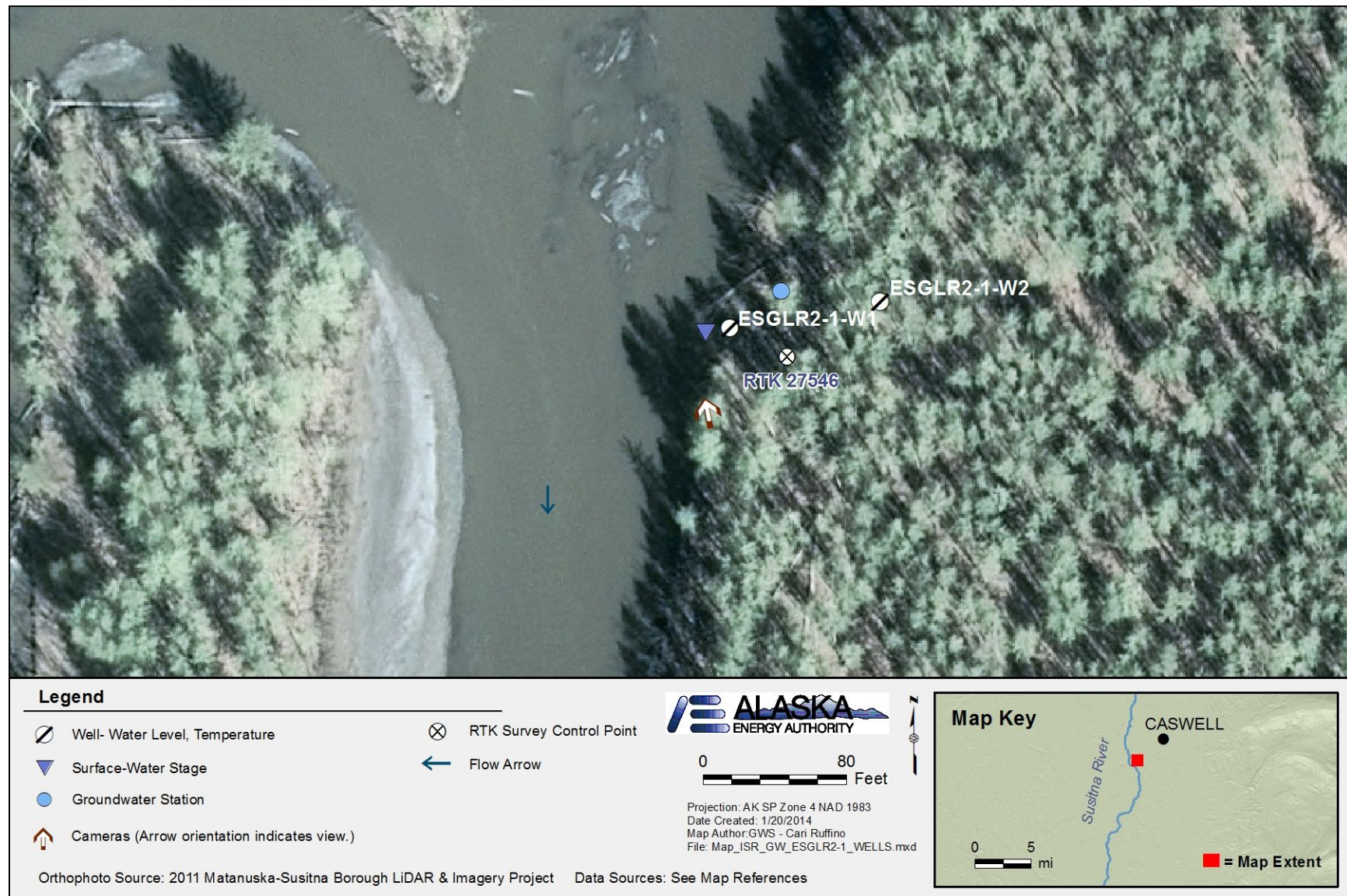
Figure 4.5-21. Well locations and continuously measured parameters at Lower River Transect Groundwater Station ESGLR2-1.
