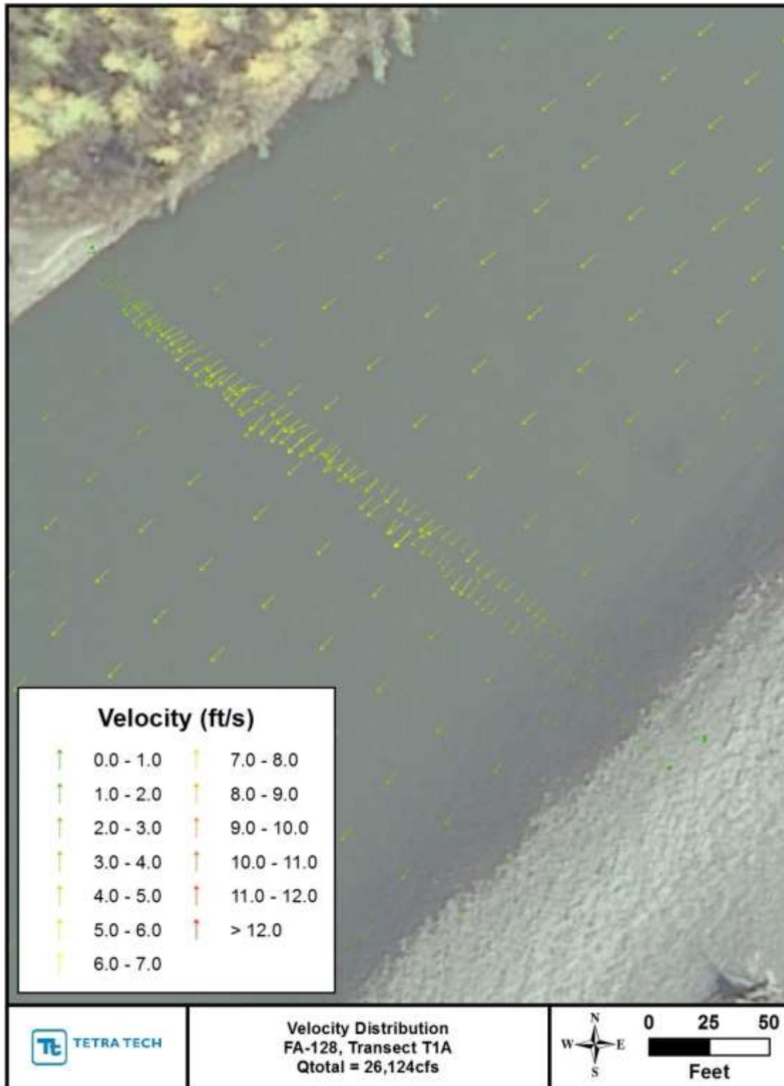
Figure 2.3-22. Comparison of measured and predicted velocity magnitude and direction at Transect 1A at 26,184 cfs (Sep 10, 2013).
