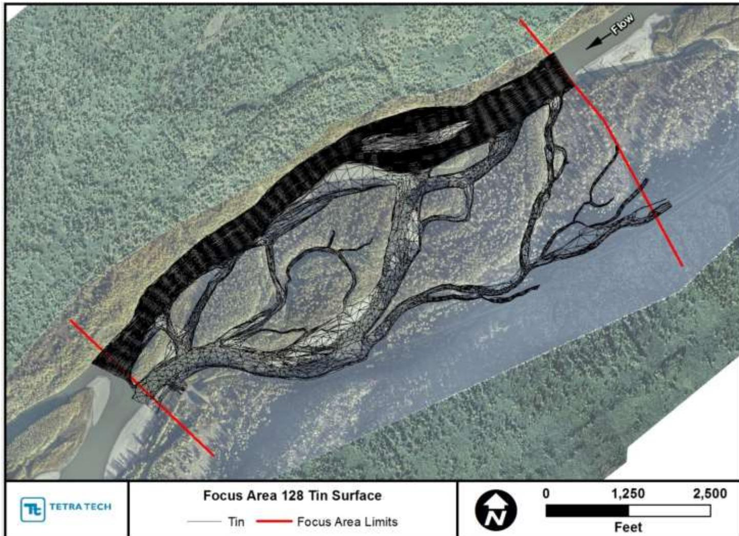
Figure 2.2-2. Triangulated Irregular Network (TIN) developed for the in-channel areas of FA-128 (Slough 8A) using the topographic and bathymetric data shown in Figure 2.2-3.
