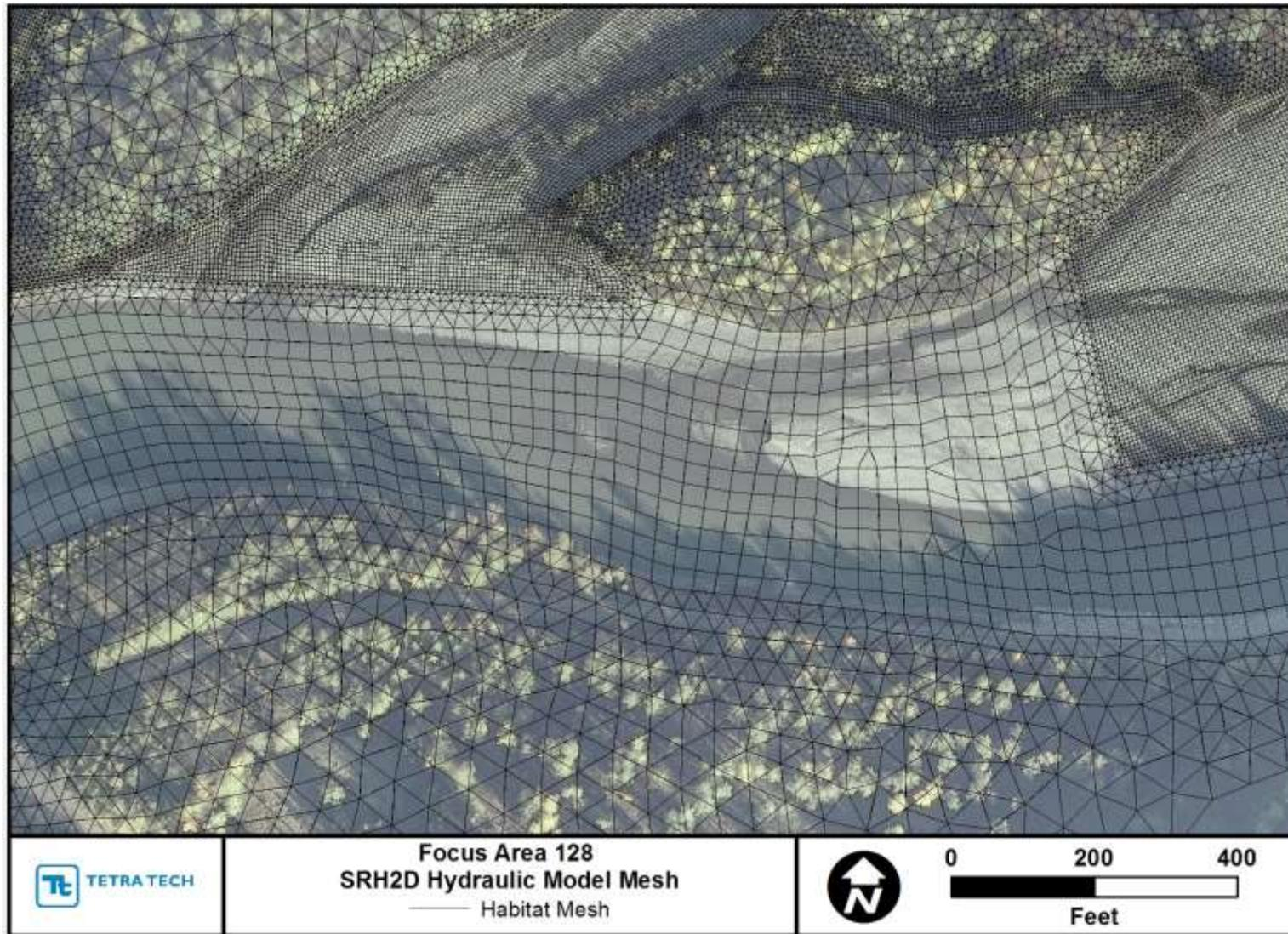
Figure 2.2-7. Close-up of a portion of the FA-128 (Slough 8A) SRH-2D hydraulic model mesh.
