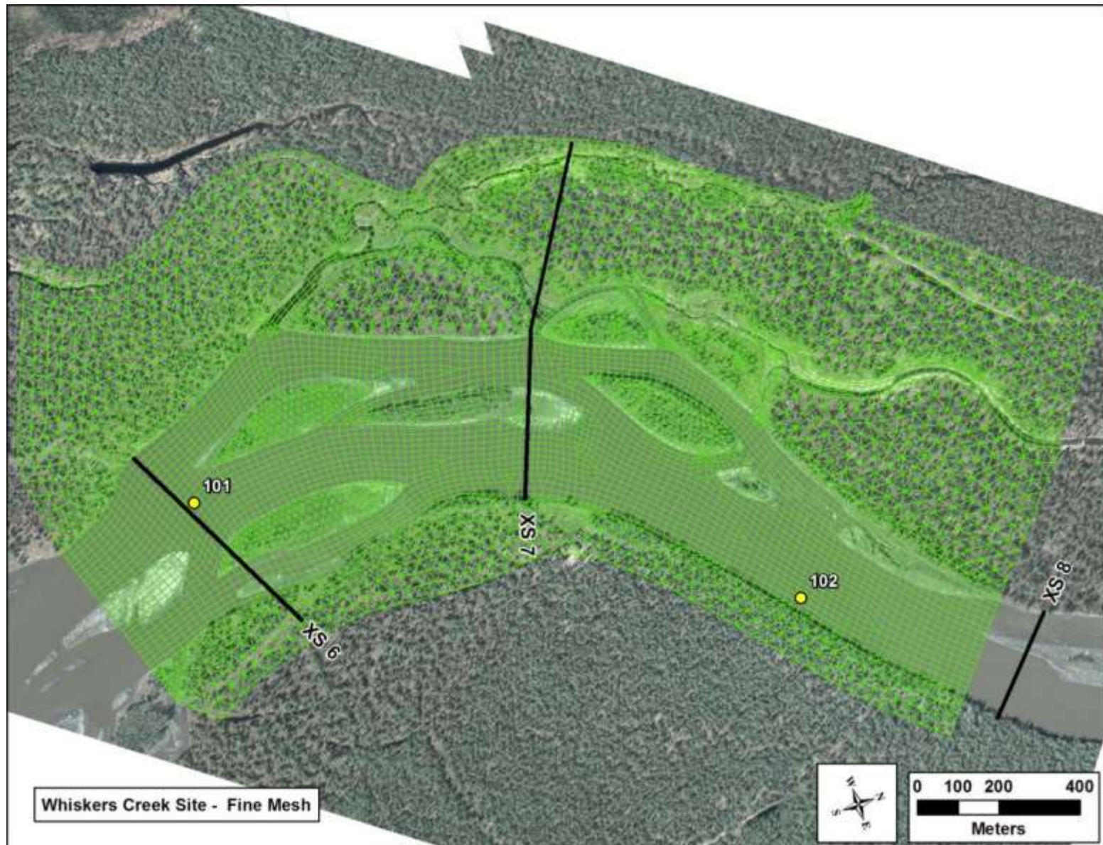
Figure 4-21. Example of Fine Mesh Applied in FA-104 (Whiskers Slough).
