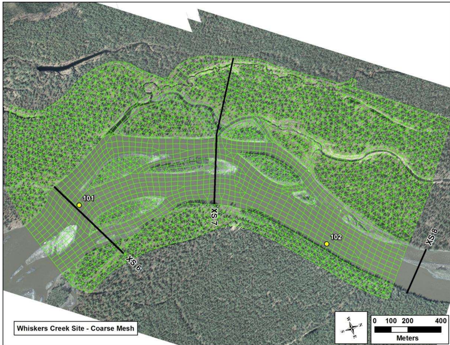
Figure 4-22. Example of Coarse Mesh Applied in FA-104 (Whiskers Slough).
