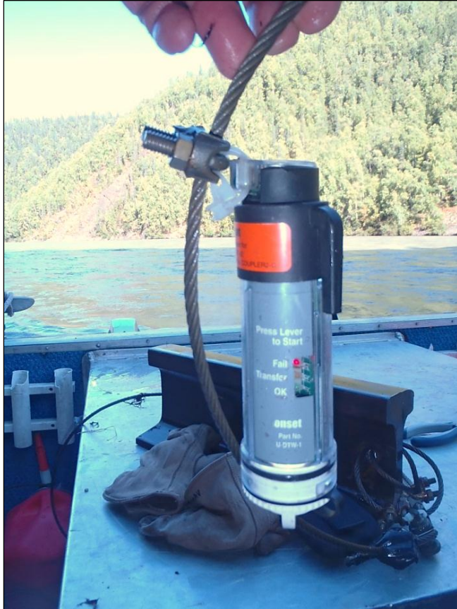
Photo A-19c. Downloading Tibit thermistor with ONSET data shuttle
