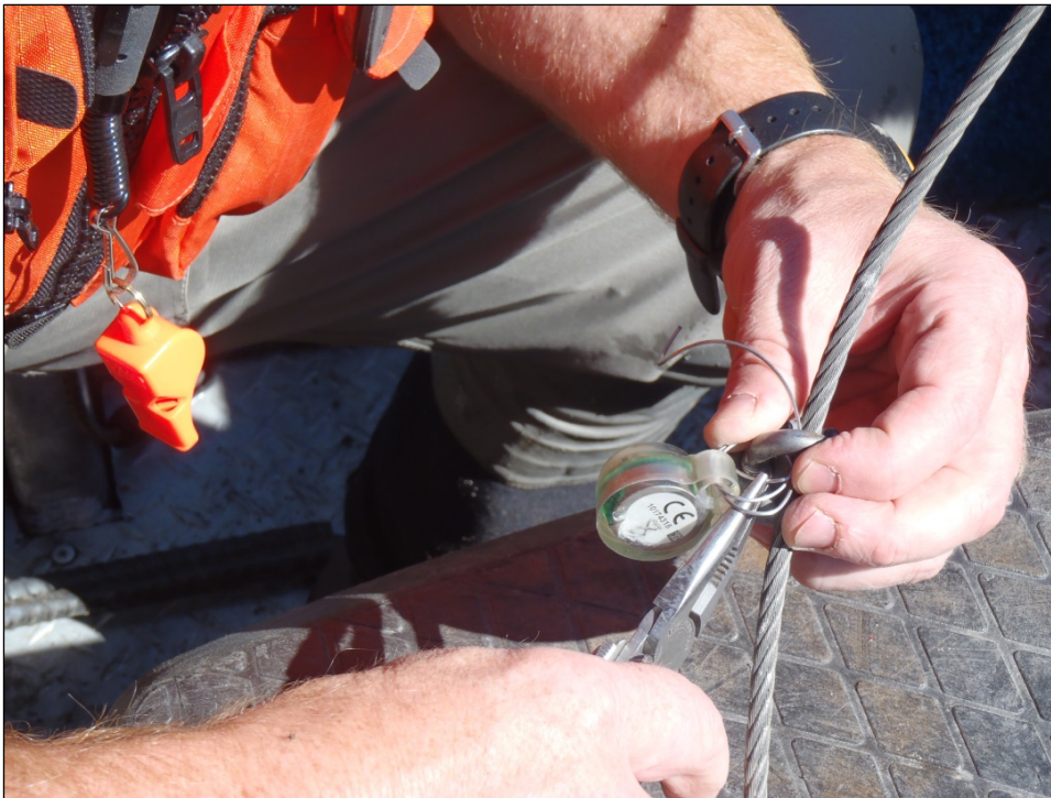
Photo A-32c. Attaching Tidbit temperature data recorder to thermistor string
