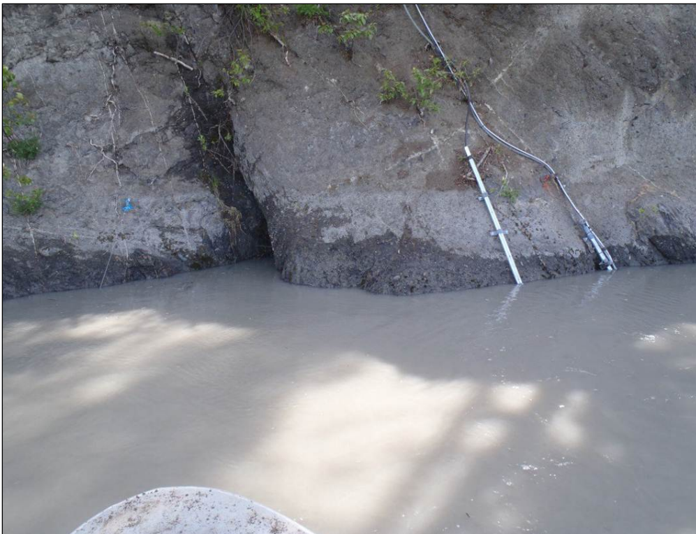
Photo A-2c. Anchor point for thermistor string on left and USGS temp monitoring equipment on right. PRM 29.9 – Susitna Station
