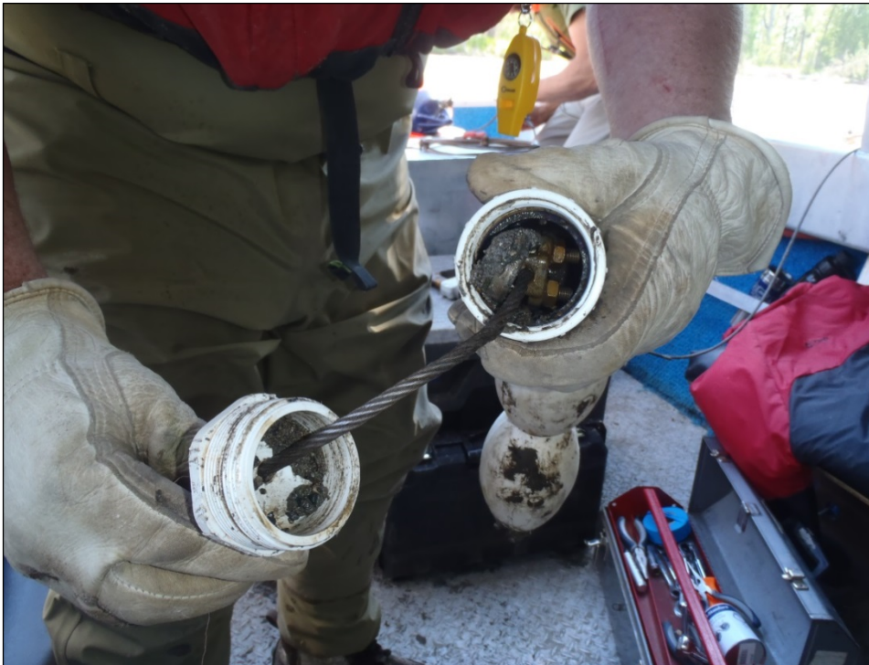
Photo A-10c. Retrieval of thermistor from 2012 overwinter system at PRM 102.8 – Talkeetna River
