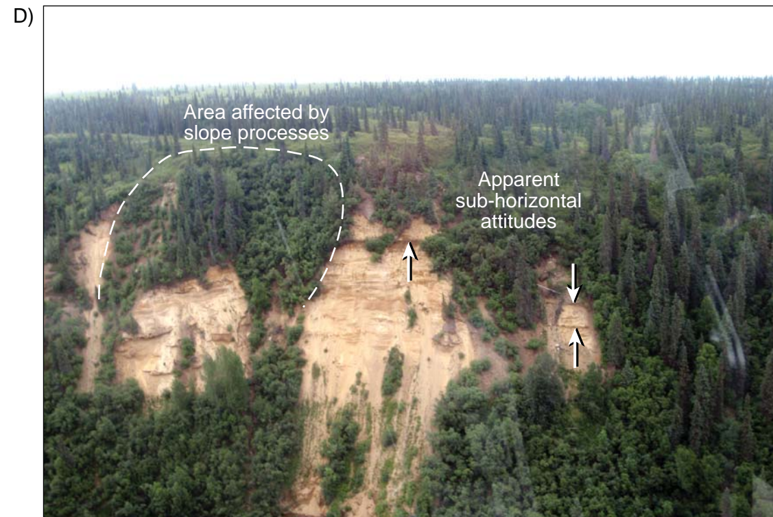
Close up view of exposure shown in Photograph (B). Note the apparently sub-horizontal basal contact between overlying till and underlying lacustrine deposits. Note sediments on the left of the image are influenced by landslide processes and not in-place locally.
