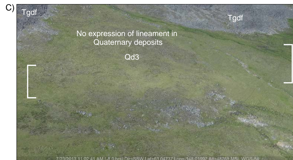
View looking west from location C. Brackets indicate the projected trace of lineament. Note absence of lineament or deformation in Quaternary deposits.
