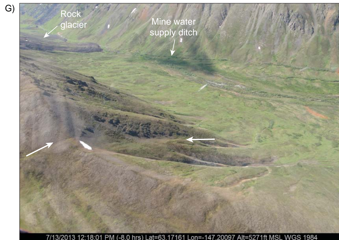
View looking southwest across an FCL-mapped lineament that corresponds to the trace of mapped Black Creek fault marked by a rock contrast. Note that no expression of faulting exists along trend in the glacial sediments of the valley floor.
