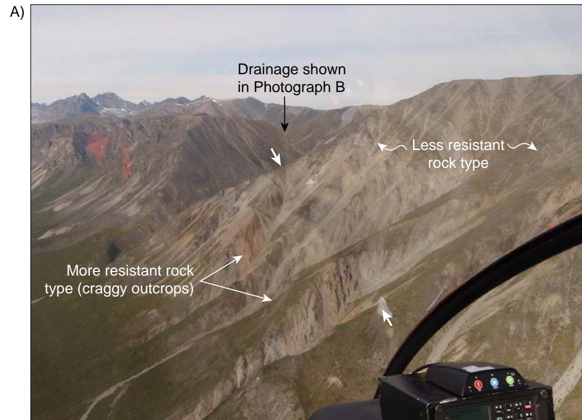
Photograph taken from location A looking southwest along apparent rock type contrast (contact?) and towards mapped lineaments in steep-walled, v-shaped, linear drainage. Arrows point along apparent contact between less-resistant rock on the north and more resistant and craggy outcrops on the south.
