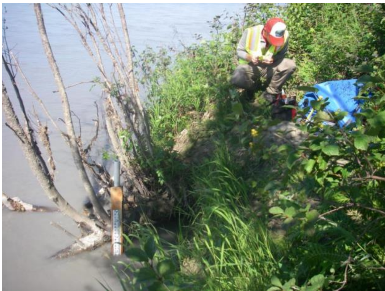
Figure 2. Example stilling well and staff gage setup.
