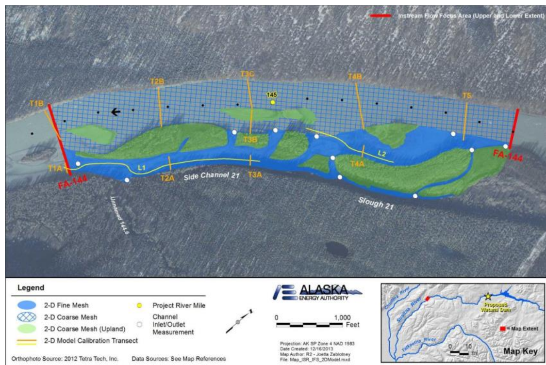
Figure 24. 2-D Model Flow Measurement Locations – FA-144 (Slough 21).
