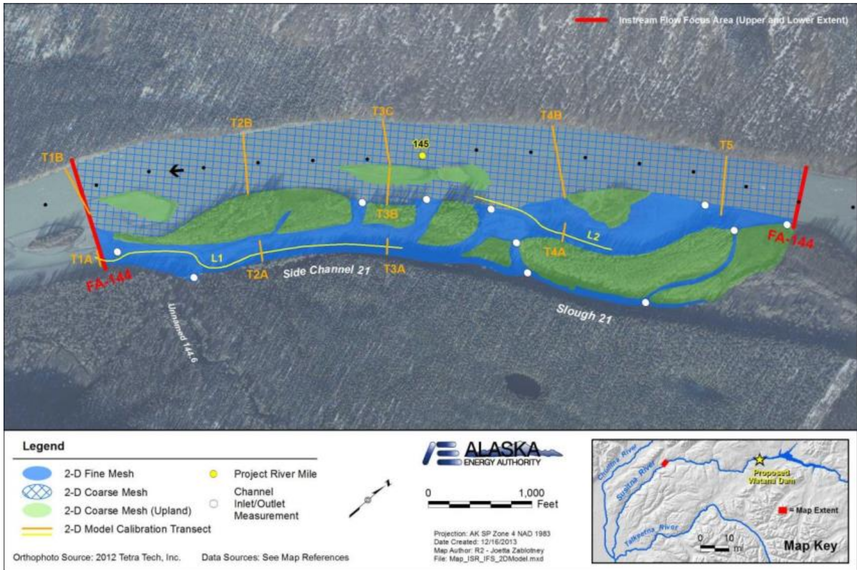
Figure 5.6-7. FA-144 (Slough 21) showing fine and course mesh overlays, channel inlet and outlet measurement locations, and alignment of 2013 calibration transects.
