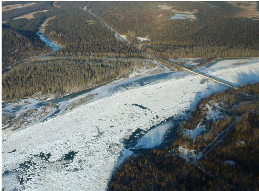
Figure 5.2.1-4. Parks Highway Bridge at PRM 88 (RM 84) on November 7, 2012 after ice cover progression through the reach. Note flooded gravel bars on both sides of the river.
