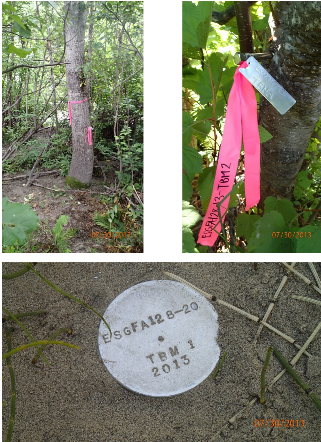
Figure E-5. This figure depicts example survey control points established at FA-128 (Slough 8A) for conducting level-loop vertical elevation surveys. The top images illustrate elevation survey temporary benchmarks (TBM) located on trees. The top right image displays TBM 2 at ESGFA128-13. The bottom image displays an aluminum cap (Alcap) on rebar (TBM1) at ESGFA128-20. It is common for rebar TBMs to frost heave in winter, so it is beneficial to use 3 to 4 points in trees or other solid features. TBMs also have to be found in the winter, which becomes difficult when there is 3 to 6 feet of snow on the ground.
