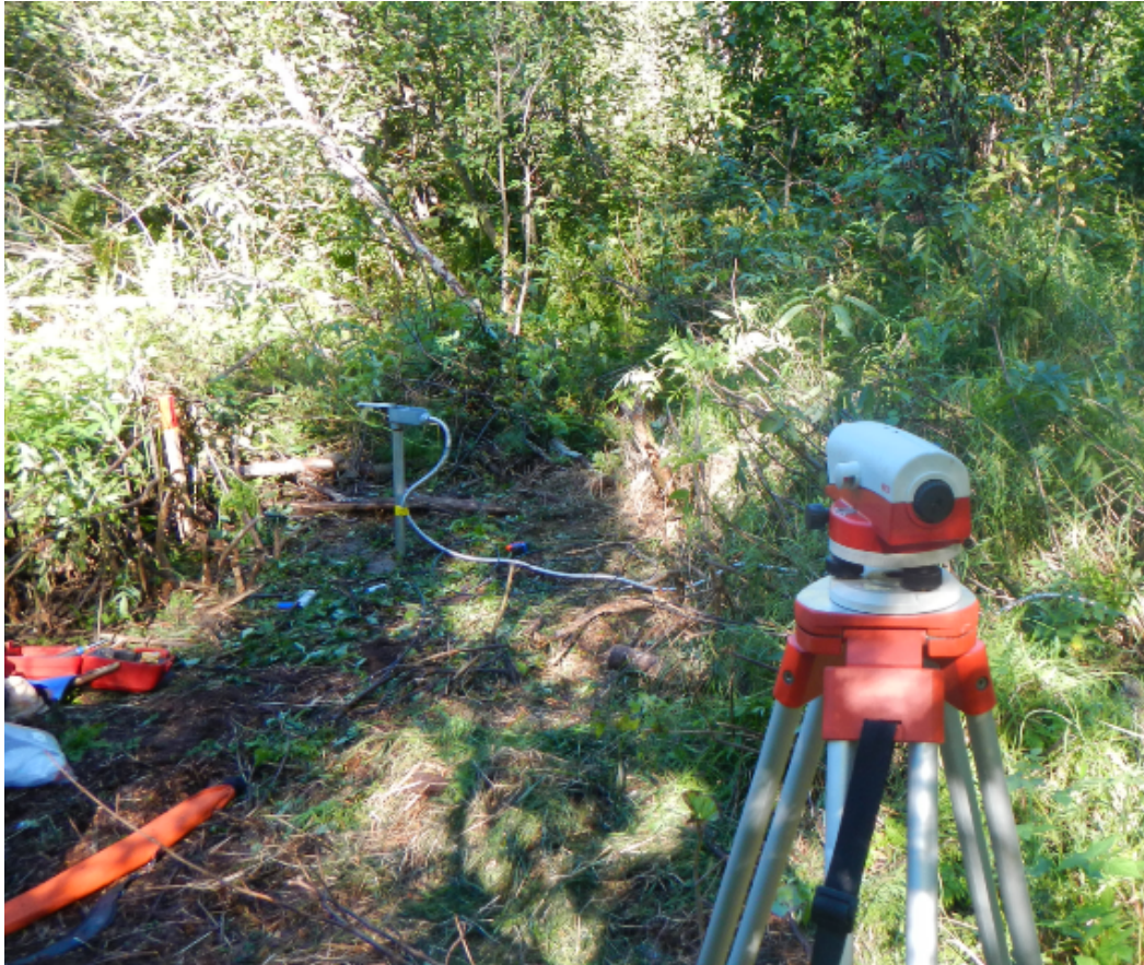
Figure E-1. This image taken at FA104 (Whiskers Slough) depicts a survey underway during a well installation to measure water levels to Project datum and accuracy standards on August 27, 2013.
