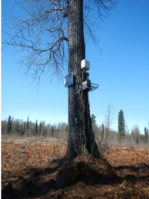
Figure 4.6-1. Image from FA-104 (Whiskers Slough), surface-water station ESSFA104-1. In many of the study area locations, flooding is an annual event with ice jam flooding producing the highest water levels. Ice jam scars on trees were used to determine the past high flood elevations. The station was installed on the Cottonwood tree about 3 feet above the highest observed ice scars in trees in the general area
