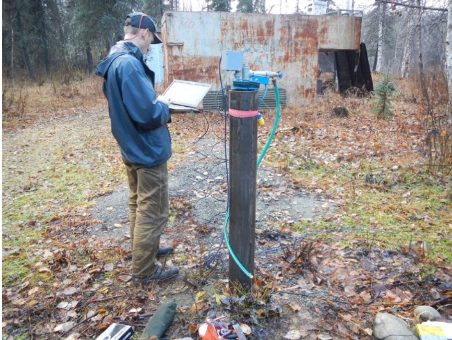
Figure 5.9-1. Example of a home owner well that has had a self-logging pressure transducer added, which record water level and temperature. This well is in FA-138 (Gold Creek) Focus Areas and adjacent to Slough 11. It is groundwater station ESGFA138-HW3. Data is only accessible during site visits.
