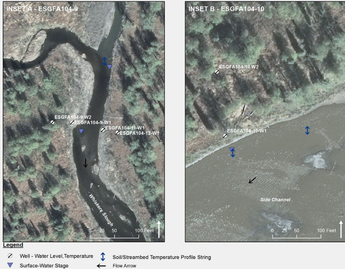
Figure 4.5-19. Inset A (left) and B (right) show locations of aquatic transects with continuously measured parameters at FA-104 (Whiskers Slough) Focus Area. These study sections are intended to improve the understanding of GW/SW interaction processes relevant to aquatic habitat evaluations.
