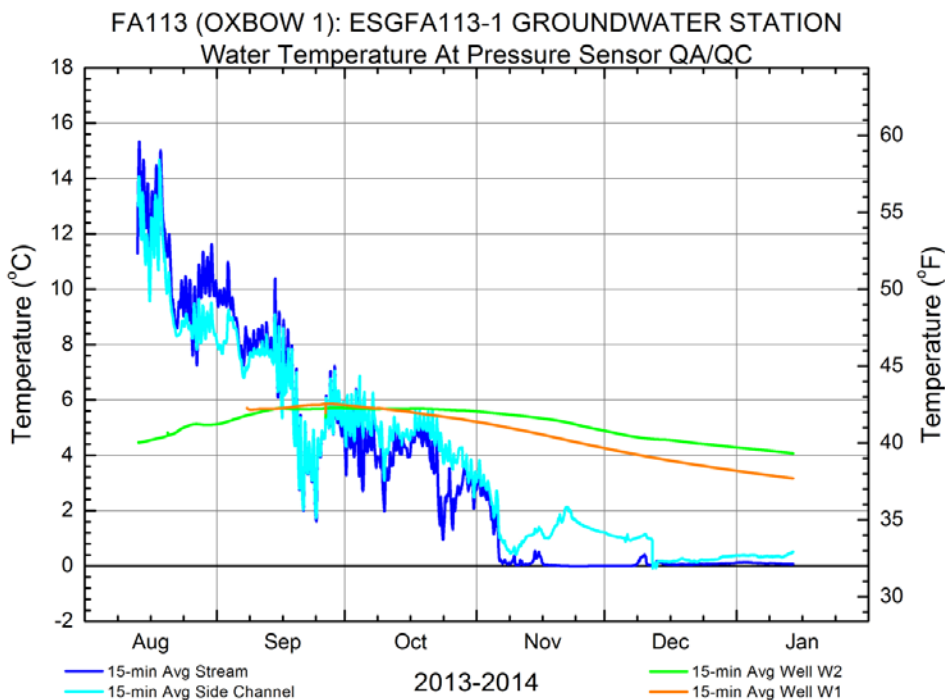
Figure 5.7-1. Example of water temperature in groundwater and surface water in the Aquatic Transect in FA-113 (Oxbow 1) from groundwater station ESGFA113-1.
