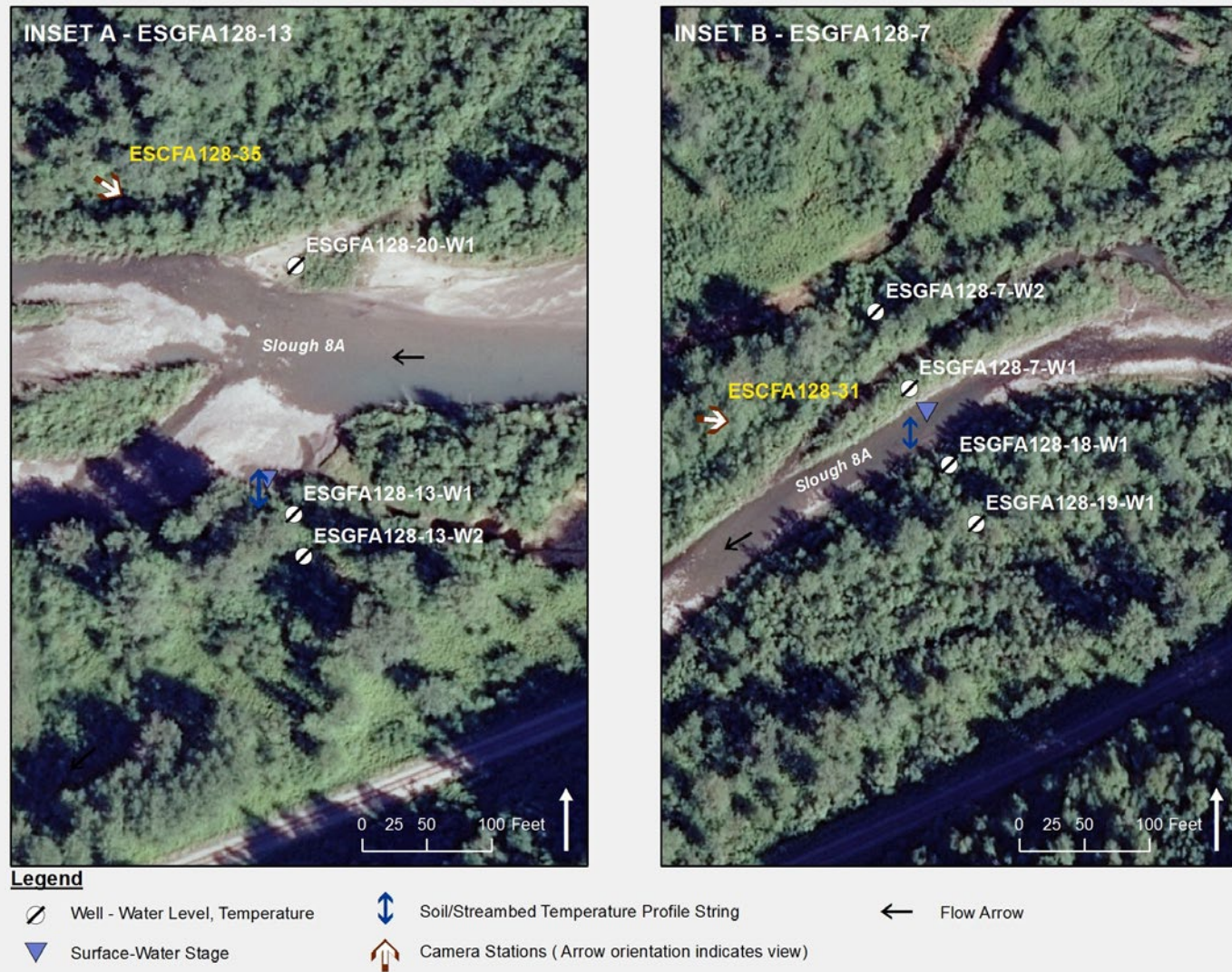
Figure 4.5-15. Inset A (left) and B (right) show locations of aquatic transect stations with continuously measured parameters at FA-128 (Slough 8A) Focus Area. These study sections are intended to improve the understanding of GW/SW interaction processes relevant to aquatic habitat evaluations.
