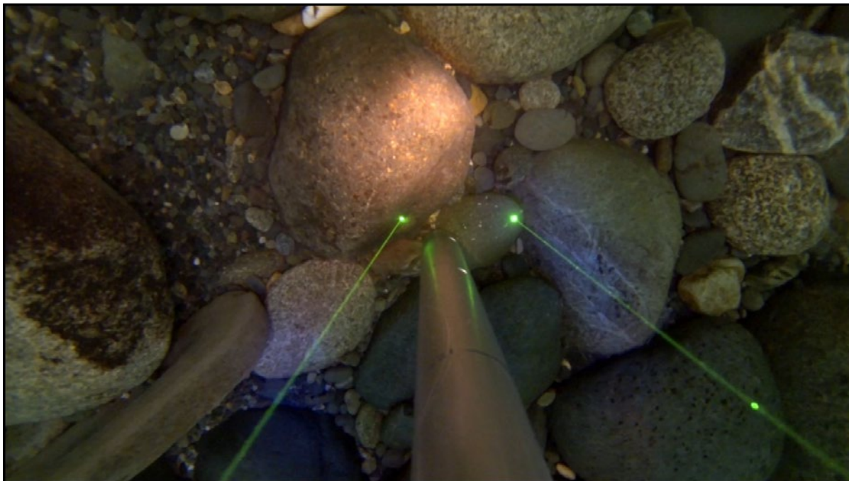
Figure 3-9. GoPro image from ESS40 using lasers and both the AquaVu integrated lights and Princeton Tec scuba flashlights.
