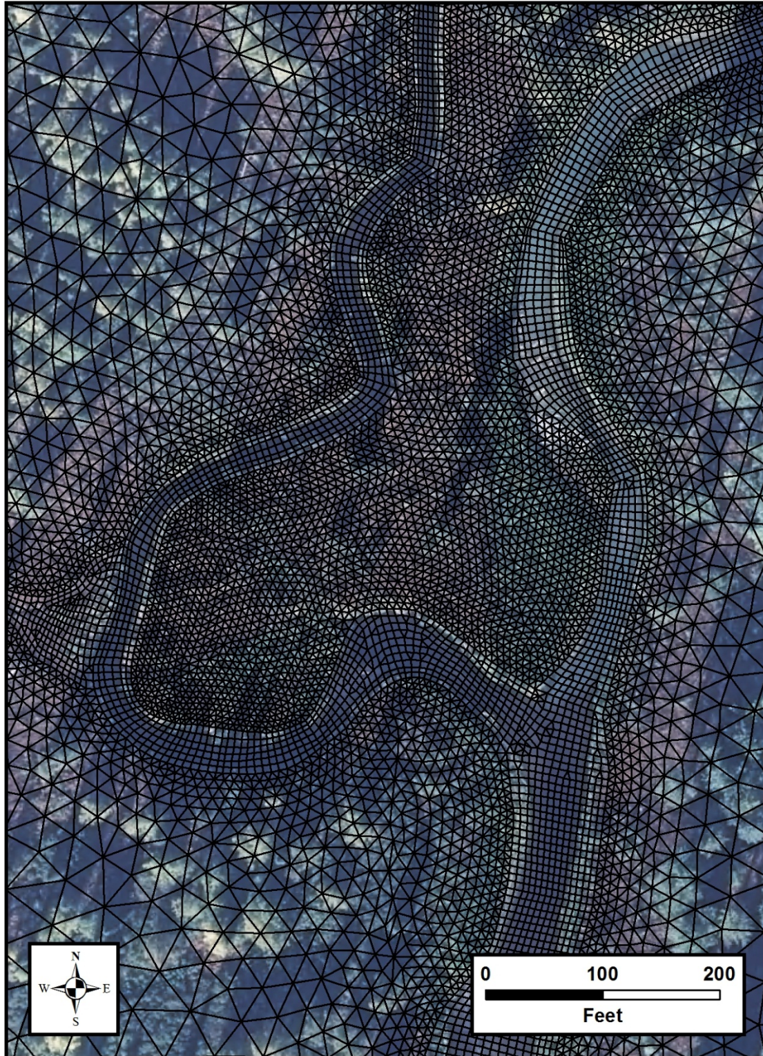
Figure 5.1-16. Example of SRH-2D Mesh in Habitat Area at the Mouth of Whiskers Creek (in FA-104) Selected to Have a Fine Mesh Size (2 meters).
