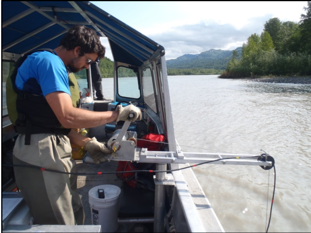
Photo I-2. Boom and hand reel used for deployment of water quality sampling equipment.
