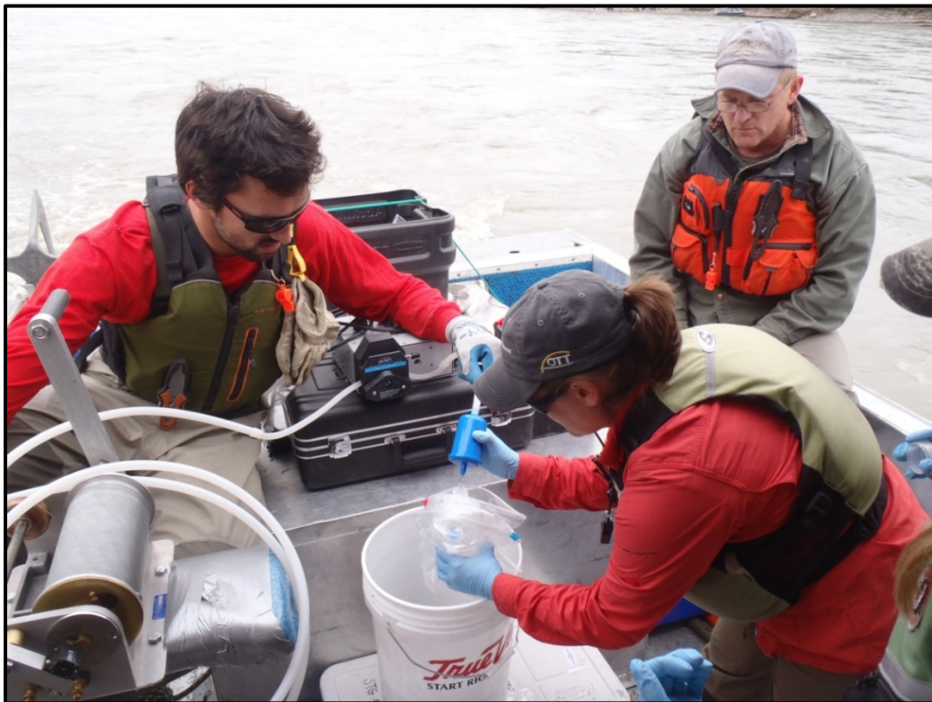
Photo I-6. Collection of filtered water quality sample.
