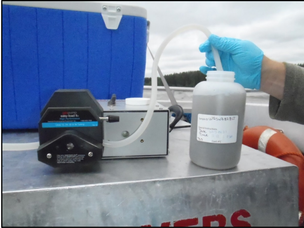
Photo I-5. Collecting non-filtered water sample using peristaltic pump
