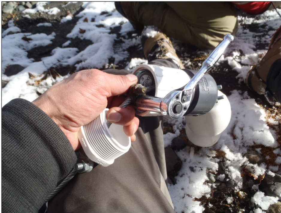
Photo A-30c. Installing thermistor in overwinter system.
