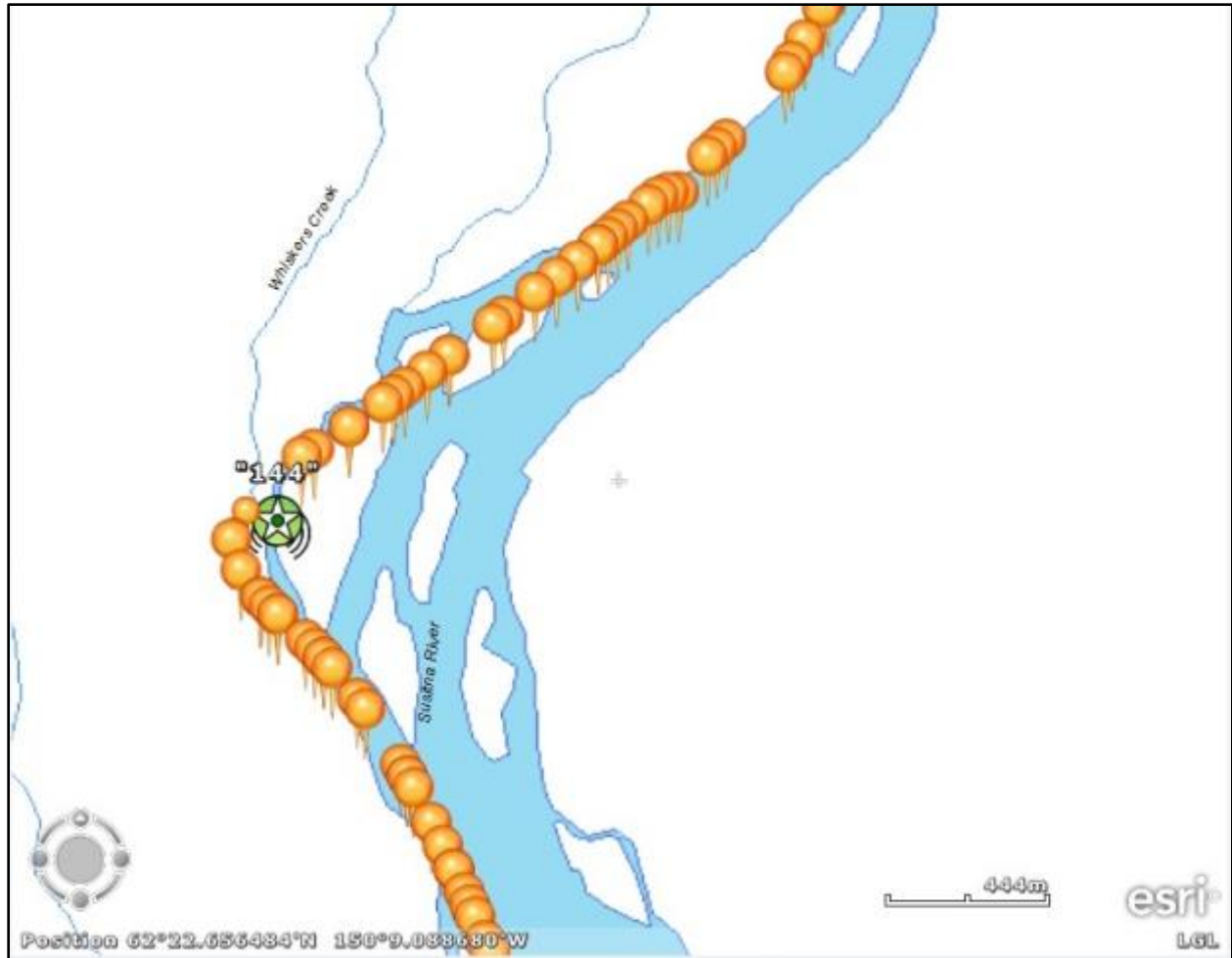
Figure C.A2-8. Detections for radio tag 151.943 Code 62 during Pass 2. The yellow circle indicates the location of the tag and the star is the location of the highest power detection. The power of the detection is located above the star and is on a scale from 40 to 154.
