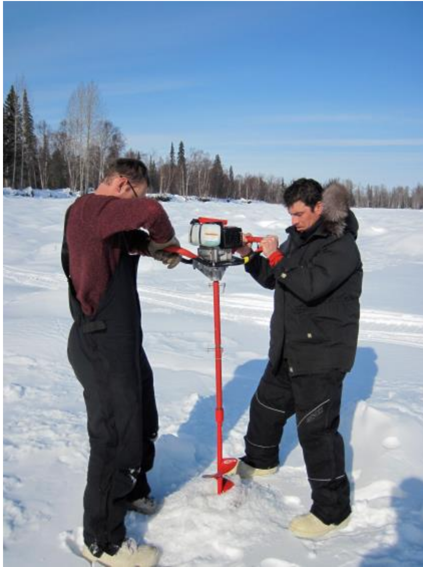
Figure C.A1-7. Drilling a hole through the ice in the mainstem Susitna River with an ice auger.
