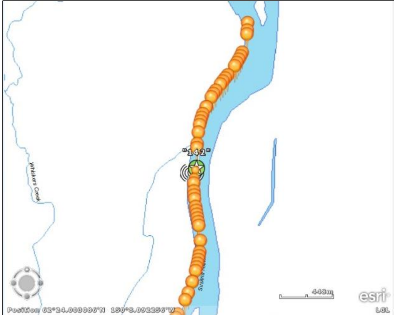
Figure C.A2-10. Detections for radio tag 151.934 Code 94 during Pass 2. The yellow circle indicates the location of the tag and the star is the location of the highest power detection. The power of the detection is located above the star and is on a scale from 40 to 154.
