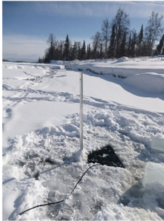
Figure C3.2-1. Photograph of the slough mouth site in FA-104 (Whiskers Slough) showing the sonar pole mount deployed in the sample hole. Water flow is from foreground towards background.
