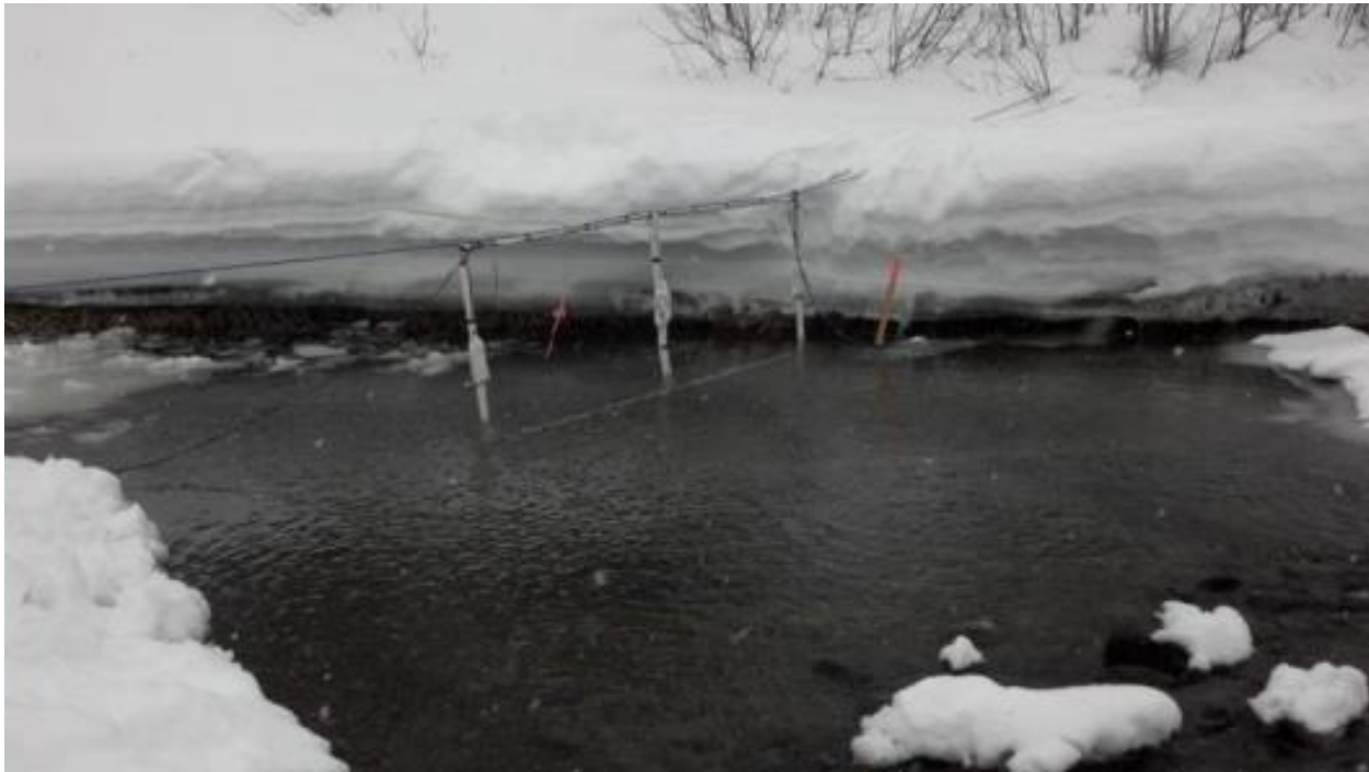
Figure C4.2-2. Swim-through test antenna repositioned in open water for comparison with through-ice performance.
