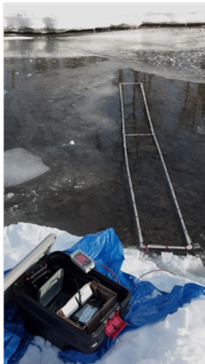
Figure C4.2-4. Swim-over test antenna used to evaluate performance of PIT antenna system (power supply, reader, data logger) in cold temperatures.
