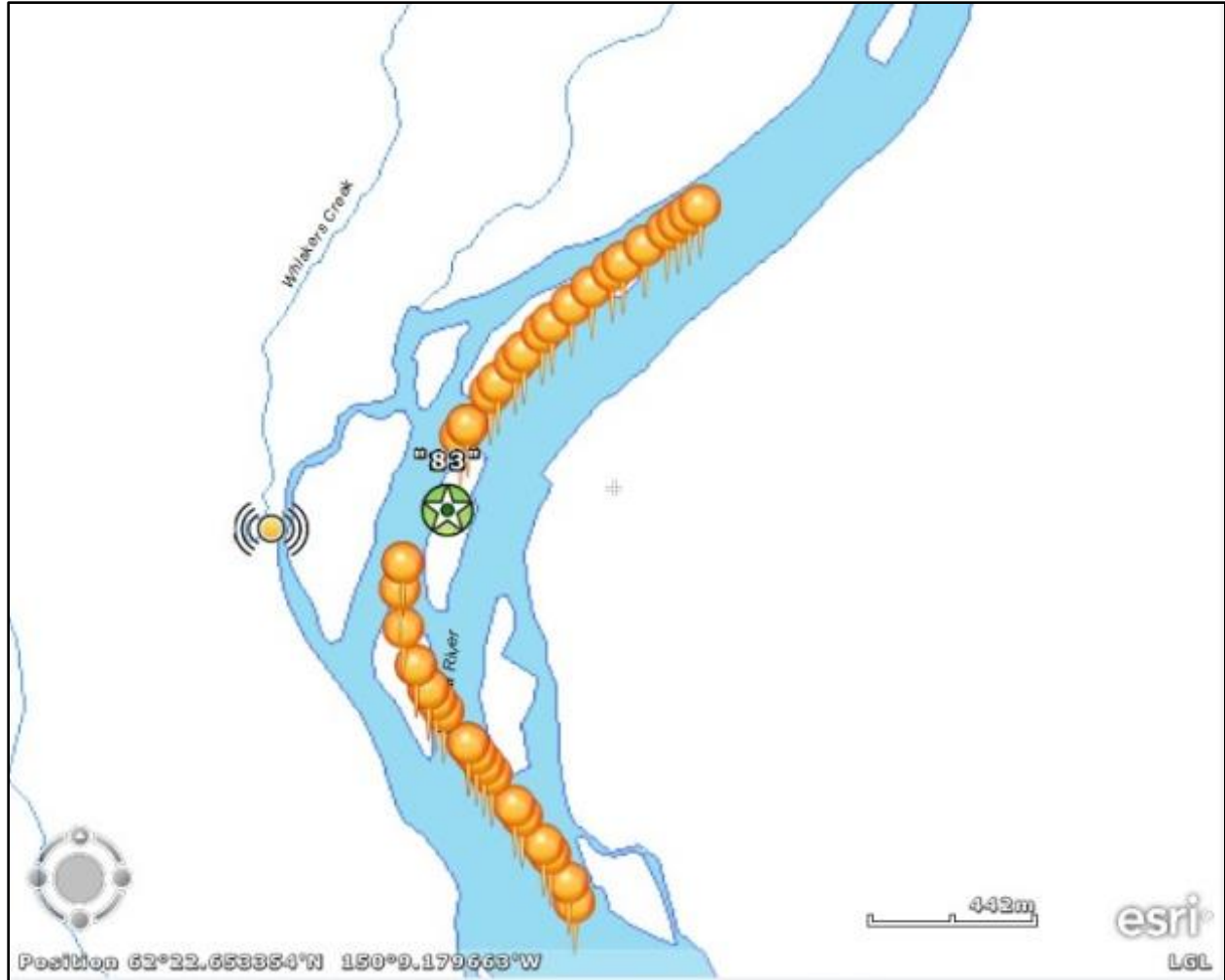
Figure C.A2-3. Detections for radio tag 151.974 Code64 during Pass 1. The yellow circle indicates the location of the tag and the star is the location of the highest power detection. The power of the detection is located above the star and is on a scale from 40 to 154.
