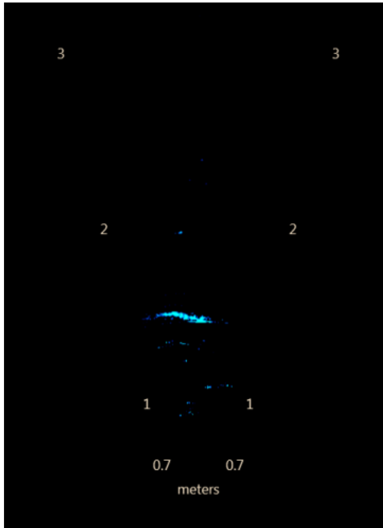
Figure C3.3-2. Truncated still image from ARIS data collected from the slough mouth site in FA-104 (Whiskers Slough) showing a single fish estimated to have a total length of 37 cm (14.5 in). A background subtraction algorithm was applied to the image to allow for better contrast of the fish against the substrate. Distance from the sonar is shown with 1 m (39 in) range increments.
