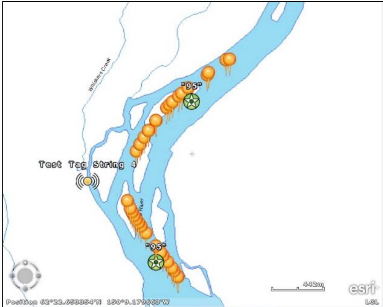
Figure C.A2-15. Detections for radio tag 151.963 Code 19 during Pass 1. The yellow circle indicates the location of the tag and the star is the location of the highest power detection. The power of the detection is located above the star and is on a scale from 40 to 154.
