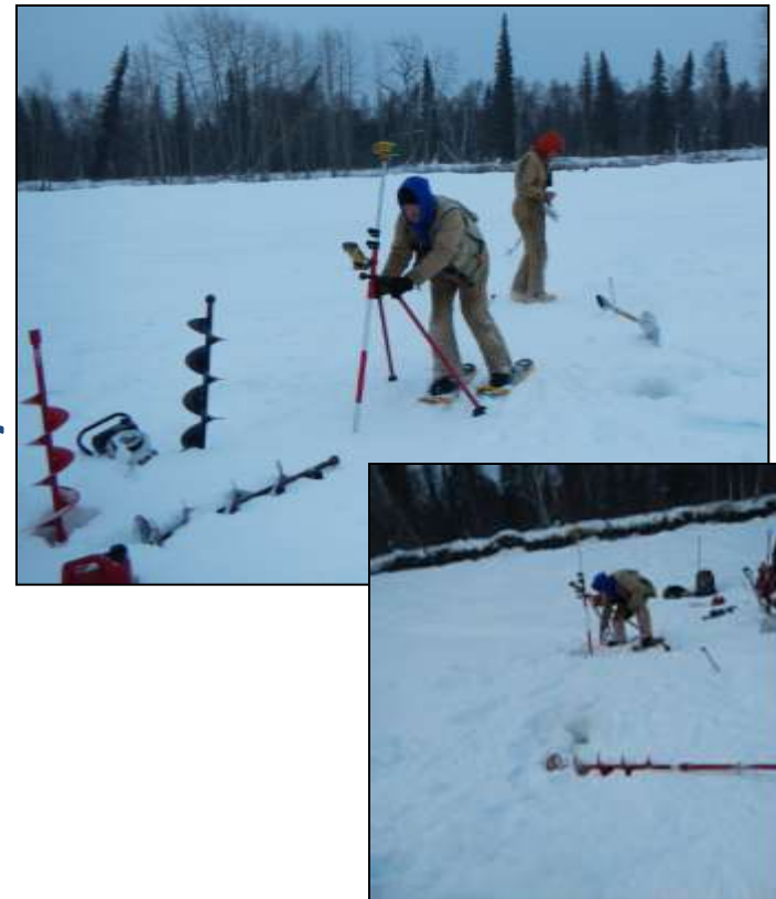
Geovera staff conducting RTK surveying at ESS40, GW Scientific and Brailey Hydrologic ice drilling, January 2013
