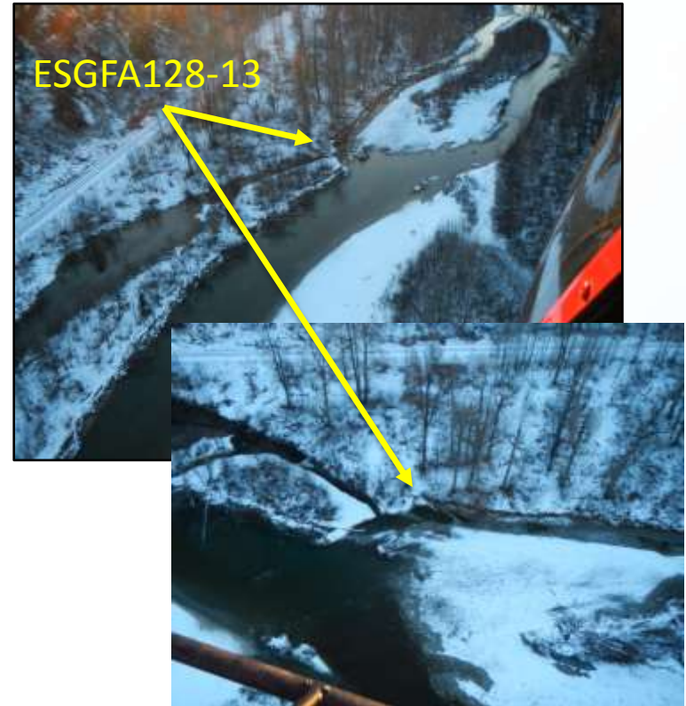
FA-128 Slough 8A, Lower Section of Slough 8A, location of ESGFA128-13 station, surface-water icing conditions are affected by groundwater upwelling, November 8, 2013
