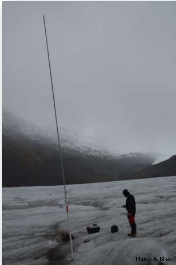
Ablation stake measurements on lower East Fork Glacier, September 2013
