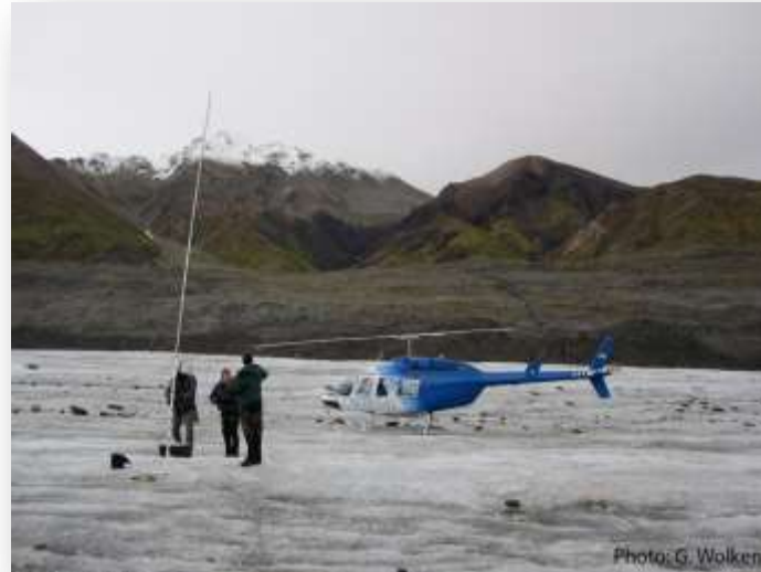
Ablation stake measurements on lower Maclaren Glacier, Sept. 2013
