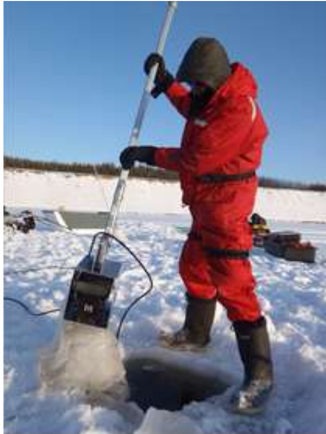
Figure 5.11-2. Photograph showing the DIDSON sonar head mounted on a bracket and fastened to an aluminum pole. The DIDSON was lowered down under the ice and used to sample fish at multiple mesohabitats in the Athabasca River in February, 2012.
