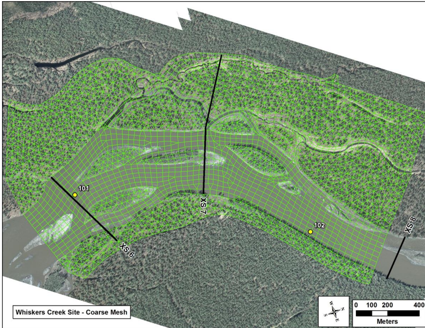
Figure 6.6-1. Example of coarse mesh applied to the Whiskers Slough potential Focus Area, Middle Susitna River Segment, Geomorphic Reach MR-8
