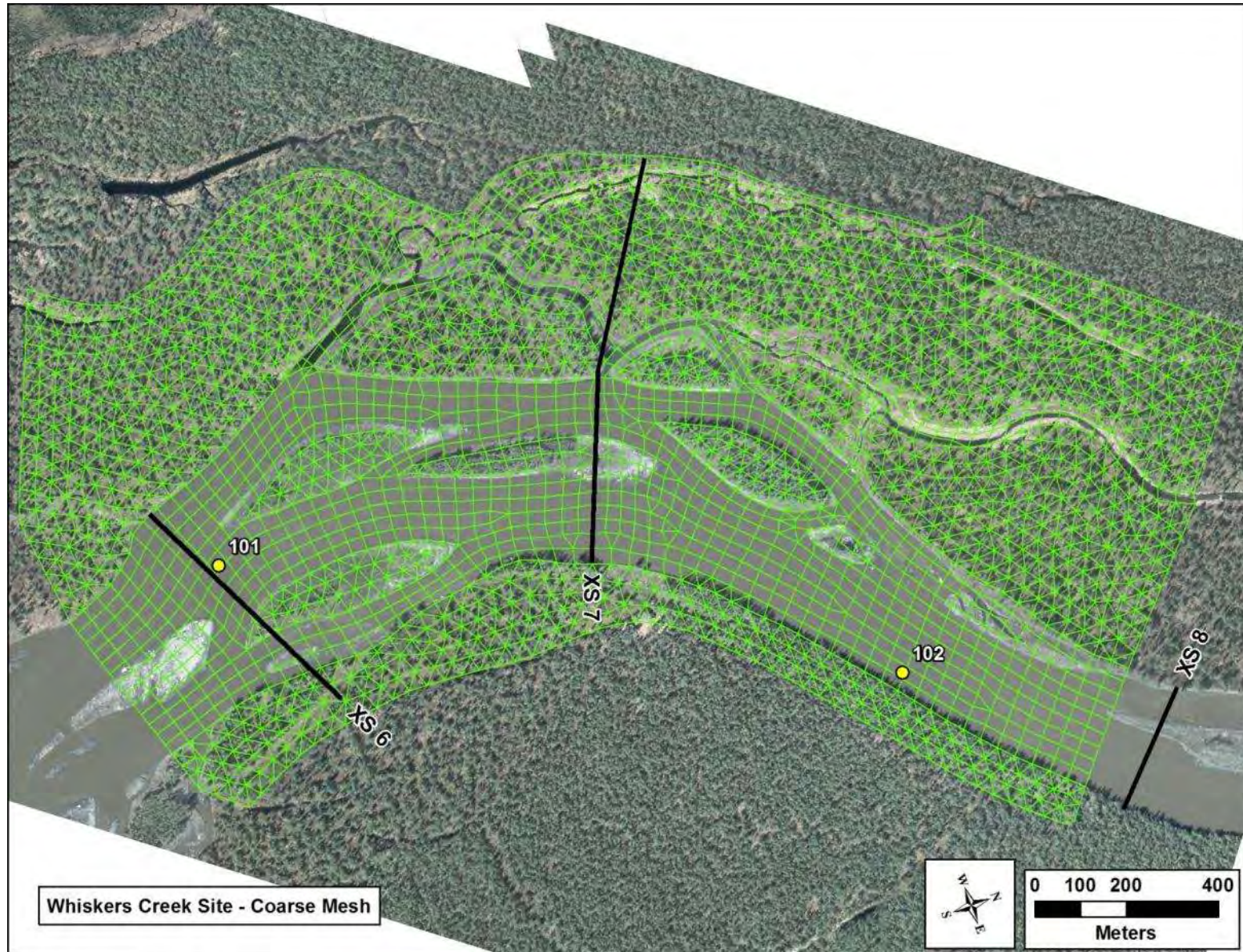
Figure 4-25. Example of Coarse Mesh Applied in Whiskers Slough Focus Area
