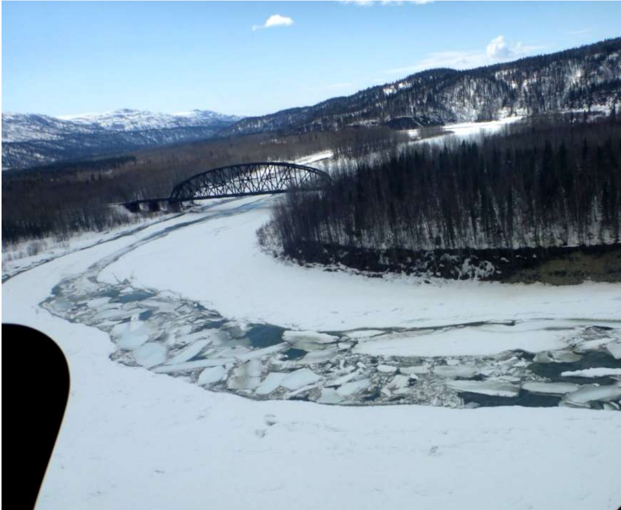
Figure 5.4-6. Velocity lead opening near Gold Creek Bridge (RM 136) on April 19, 2012. Broken ice is accumulating in the lead.
