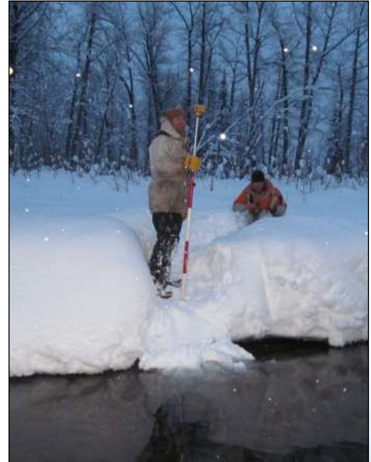
GW Scientific, Geovera establishing survey control for water level station and R2 IFS site , February 12, 2013
