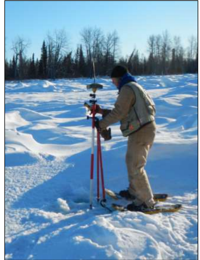
Geovera staff conducting RTK surveying at gaging station ESS40, January 2013
