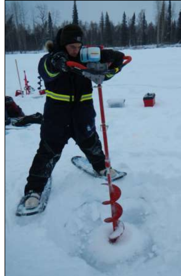
GW Scientific staff drilling ice holes for velocity measurements, upstream of gaging station ESS40, January 2013
