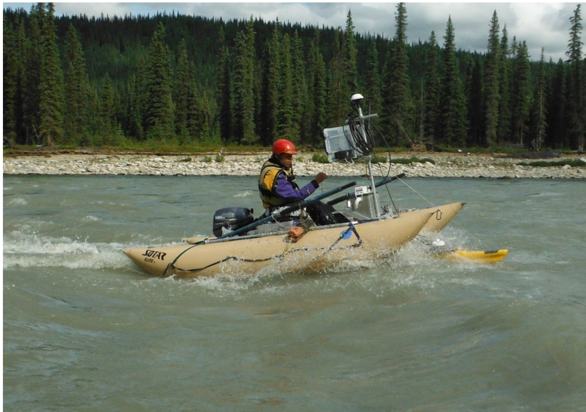
Figure 3.2-1. ADCP cataraft in 1-foot standing waves at PRM 183.5, August 7, 2012.
