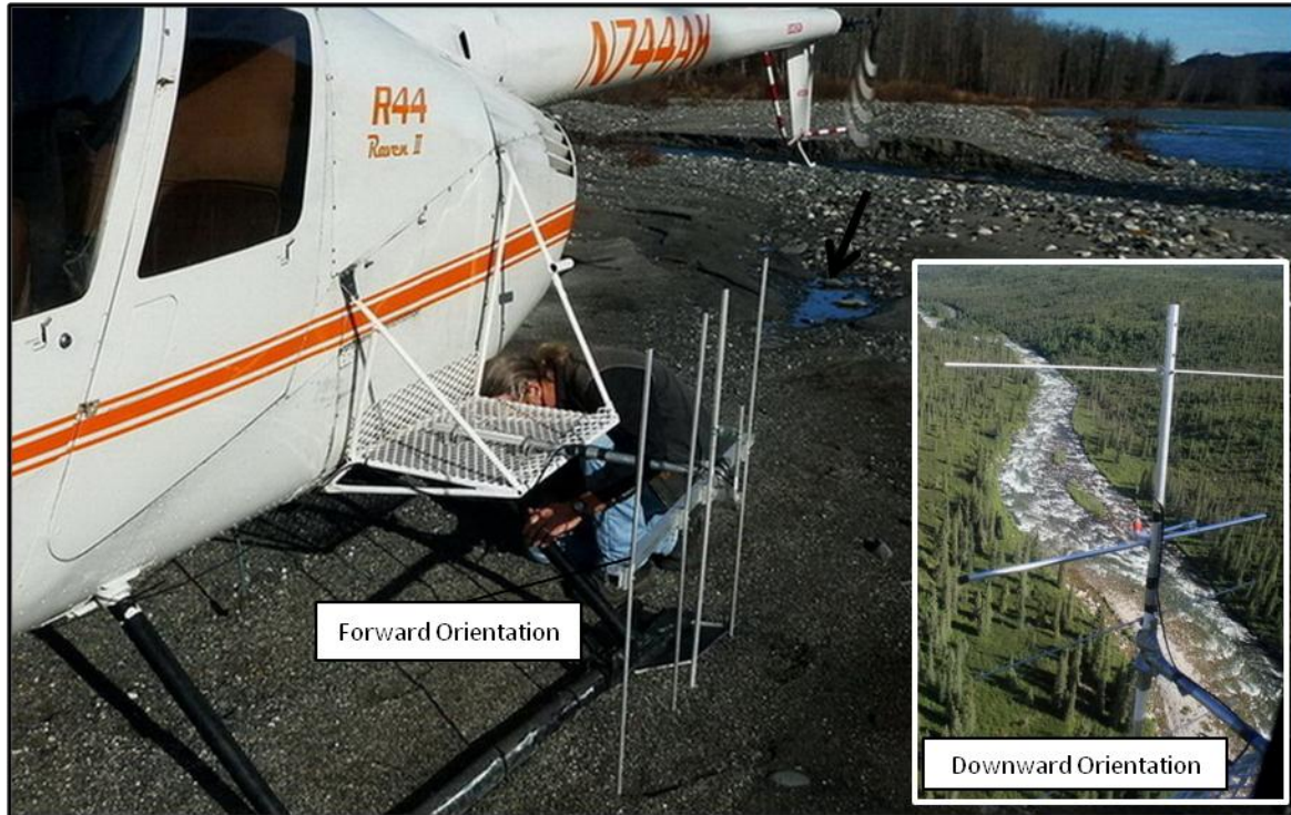
Photo 5. Helicopter (R44) setup for aerial-tracking surveys conducted on the Susitna River in 2012.
