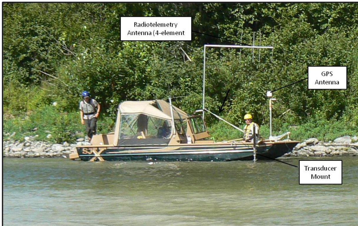
Photo 6. Setup for boat surveys using sonar to assess spawning activity in turbid water, July 28, 2012.
