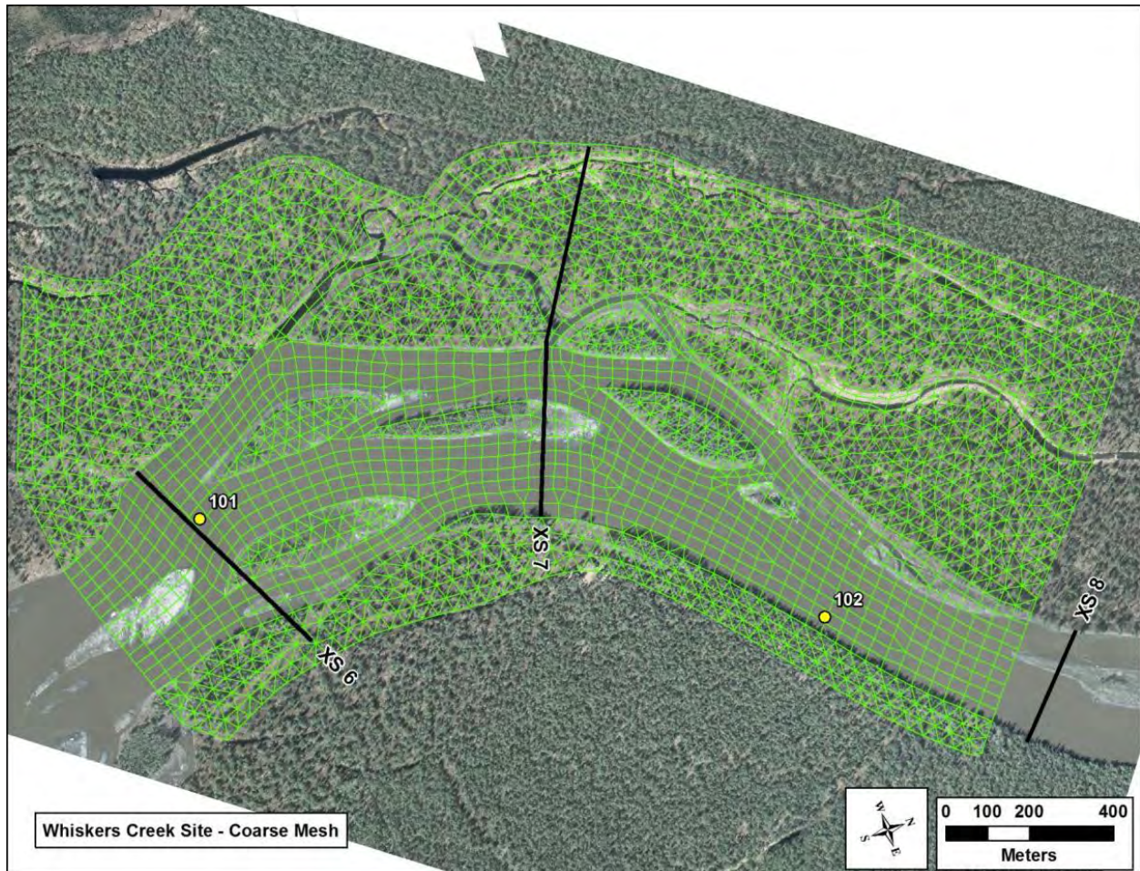
Figure 6.6-1. Example of coarse mesh applied to the Whiskers Slough potential focus area, Middle River Reach 8
